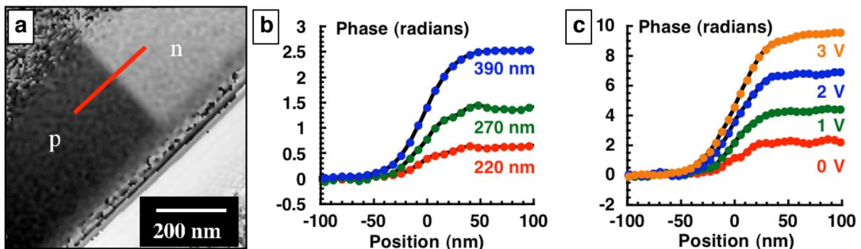
**Figure 3.** (a) Electron holographic phase image acquired from a Si p-n junction prepared for electron microscopy using focused ion beam milling. (b) Phase profiles along the line marked in (a) obtained from three unbiased specimens whose thicknesses are indicated. (c) Line profiles across a p-n junction in a specimen of thickness 390 nm, acquired as a function of applied reverse bias using a home-built electrical biasing sample holder.
