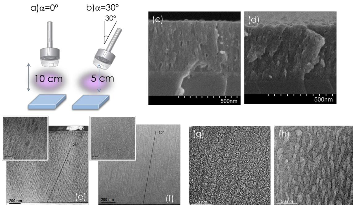
**Figure 1** – Setups used for producing the coatings studied: (a) and (b); (c) deposition at  $\alpha=0$  (setup (a)); (d) deposition at  $\alpha=30^\circ$  (setup (b)); influence of pressure on pore orientation for  $\alpha=30^\circ$ : (e)  $3.0 \times 10^{-2}$  mbar and (f)  $7.2 \times 10^{-2}$  mbar. Influence of power supplied to the target on the pore size (deposition at  $\alpha=30^\circ$  and Helium pressure of  $5.0 \times 10^{-2}$  mbar): (g) 50 W and (h) 300 W.
