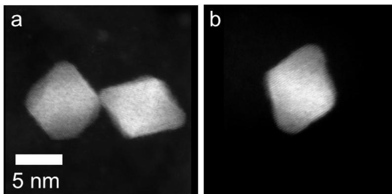
**Figure 1:** High resolution HAADF STEM images of PtNiRh octahedral nanoparticles after (a) 4 k and (b) 30 k cycles, respectively.
