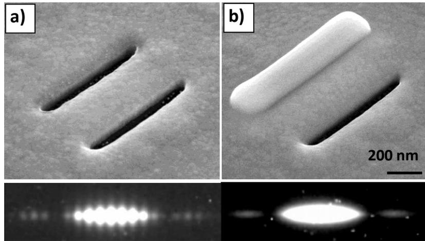
Fig. 1: Feynman double-slit experiment. (a) Two nanoslits opened by FIB milling and, below, the interference pattern of 200 keV electrons measured with TEM; (b) single-slit sample obtained by covering the left slit with a FEBID Pt layer and, below, the corresponding diffraction pattern.
