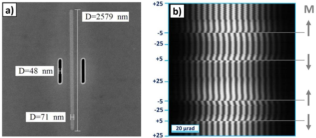
Fig. 2: Ehrenberg-Siday experiment. (a) Double-nanoslit with a Co nanowire deposited in between by FEBID; (b) interference fringes of 300 keV electrons measured with TEM as a function of the tilt angle in order to change the magnetization direction along the Co nanowire. At  $\pm 5^\circ$  magnetization reverses as shown aside by the arrows and the fringes shift abruptly.
