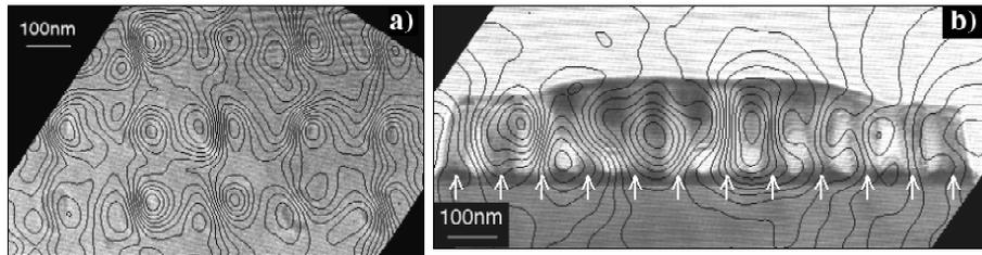
Fig. 2. Magnetic contributions to measured electron holographic phases for remanent states of a) Co dots (contour spacing 0.033 radians) and b) Ni pillars (arrowed, contour spacing 0.05 radians). The contour spacing is inversely proportional to the in-plane component of the magnetic induction integrated in the incident beam direction. Note the strong interactions between the Ni pillars, which were initially thought to be perpendicularly magnetised, and the magnetic domains within them.
