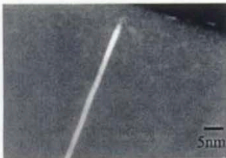
Fig. 3. 200 dark field image showing the Al-rich quantum well.
