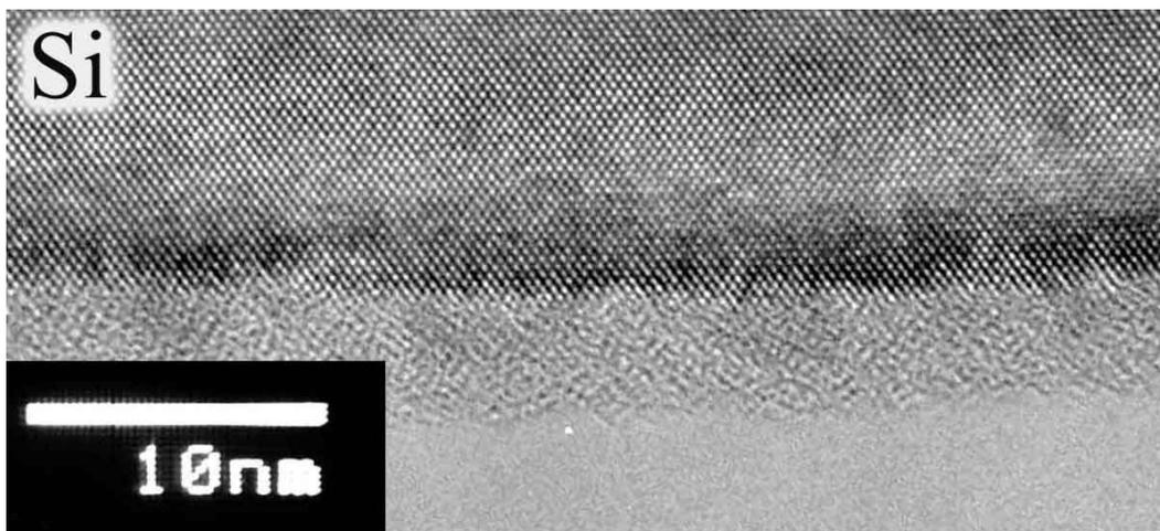
**Figure 3.** High resolution image taken on the above sample after low energy Ar ion bombardment. The damage is reduced substantially.
