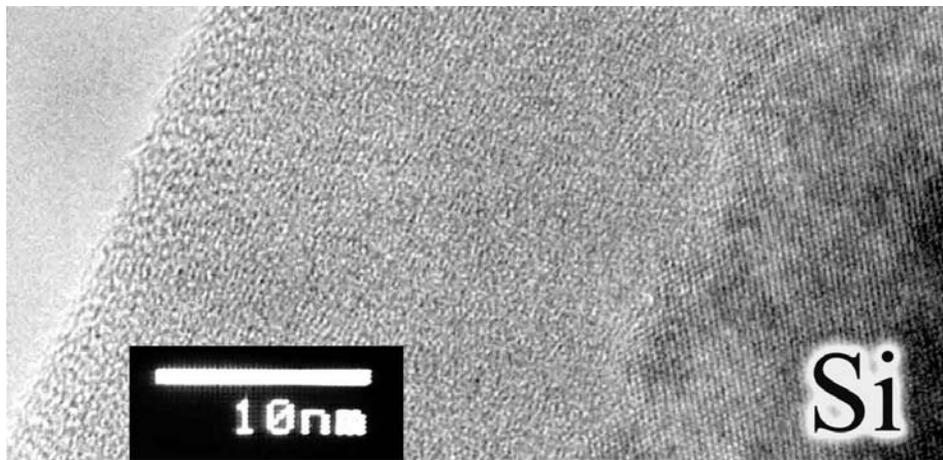
**Figure 2.** High resolution image taken on the Si sample after FIB preparation. Thick amorphous coverage is evident from the image taken at the edge of the sample.
