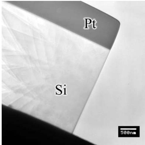
**Figure 1.** Overview of the sample after FIB preparation.
