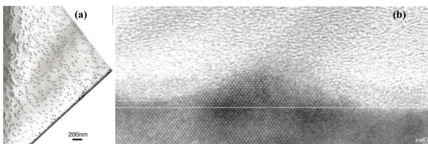
Fig. 1. (a) [001] zone axis bright-field plan-view TEM image of uncapped QDs grown with 1.75 ML InAs deposited at a growth rate of 0.016 MLs<sup>-1</sup>. (b) [110] zone axis HRTEM image of an uncapped QD grown with 1.75ML InAs deposited at a growth rate of 0.016 MLs<sup>-1</sup>.
