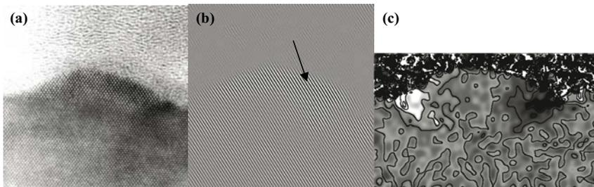
Fig. 3. (a) [110] cross-sectional HRTEM image of a smaller InAs QD with 2.7 ML InAs deposition. (b) reconstructed image by inverse Fourier transformation using the sideband  $\bar{1}\bar{1}\bar{1}$ , a misfit dislocation is indicated by arrow, (c) a lattice rotation contour map measured for the QD shows two dislocations formed at the QD edges.
