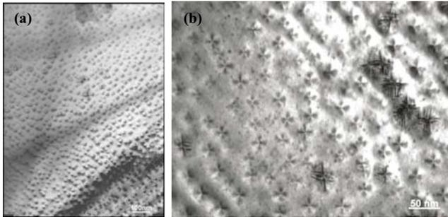
Fig. 2. (a) [001]-zone bright-field TEM image of uncapped QDs grown with 2.2ML InAs deposited at a growth rate of  $0.016 \text{ MLs}^{-1}$ . (b) [001] plan-view bright field TEM image of uncapped QDs with 2.7ML of InAs deposition.
