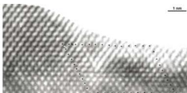
Fig. 4. [110] cross-sectional HRTEM image of an unburied QD. The black dotted line shows the determination of Burgers vector.
