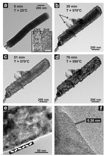
FIG. 1 (a) Bright-field TEM image of a thick, low-aspect-ratio Zn0.92Ga0.08S@CNT. Inset: detail of the sulphide core – carbon shell region. Scale bar: 2 nm. (b) to (d) Different stages of the structure during in-situ TEM oxidation. The arrows in (b) indicate unexpected foreign structures. (e) Detail of (d) highlighting the faceted nature of the thick external wall. (f) High-resolution image of an oxide grain on the external wall of (d).
