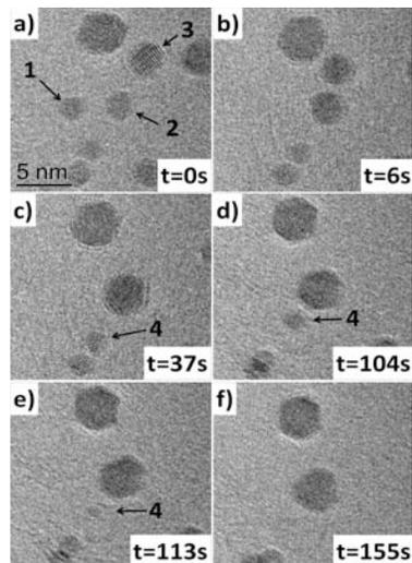
FIG. 3. Au particles on a BN support imaged in 130 Pa of  $H_2$  at  $410^\circ C$  at the indicated times at 300 kV with  $C_S$  set to below  $5 \mu m$ . The numbers refer to particles that undergo different sintering mechanisms.
