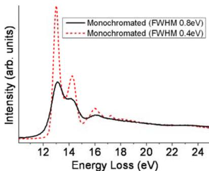
FIG. 4. Non-monochromated and monochromated EELS spectra acquired in an ETEM from  $N_2$  gas.
