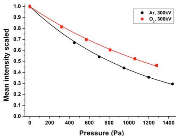
FIG. 5. Normalized image intensity in vacuum (with no specimen present) measured as a function of gas pressure for Ar and  $O_2$  at 300 kV.
