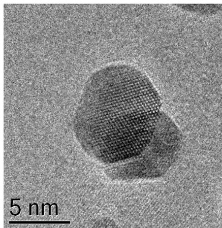
FIG. 2. High-resolution TEM image of Au particles on a BN support imaged in 320 Pa of  $O_2$  at room temperature.
