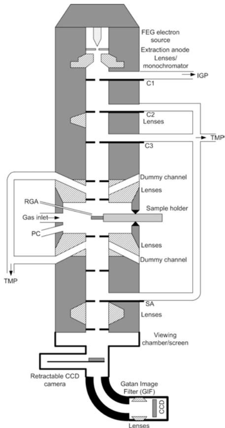
FIG. 1. Schematic diagram of a differentially pumped TEM column. FEG: field emission gun; IGP: ion getter pump; TMP: turbo molecular pump; RGA: residual gas analyzer; PC: plasma cleaner; C1: first condenser aperture; SA: selected area aperture.
