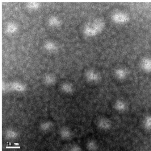
**Figure 1** Plan-view HAADF STEM image of an array of 1.65 ML InAs QDs grown on InGaAsP and covered with a 1.7 ML GaAs layer, prior to full capping with InGaAsP.
