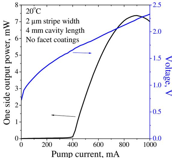
**Figure 4** CW light-current (black) and voltage-current (blue) characteristic of a 2 µm wide stripe QD laser (L = 4 mm) at 20°C heat sink temperature
