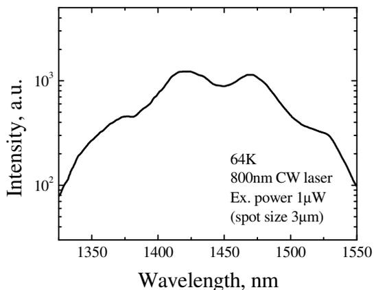
**Figure 3** PL spectrum of InAs QDs covered with 1.7 ML of GaAs taken at 64 K.
