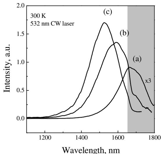
**Figure 2** Room temperature PL spectra of InAs QDs in an InGaAsP ( $Q_{1.08}$ ) matrix for different GaAs capping layer thicknesses: (a) no GaAs, (b) 1.5 ML GaAs, (c) 1.7 ML GaAs. The grey area shows the sensitivity cut-off of the detector.
