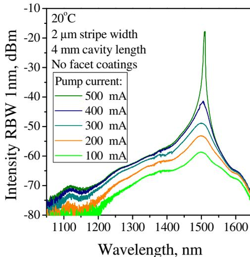
**Figure 5** EL and CW lasing spectra of a 2 µm wide stripe QD laser (L = 4 mm) at 20°C heat sink temperature.
