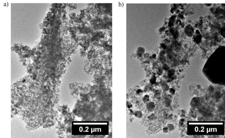
**Figure 1.** Representative bright-field TEM images of a CuSn catalyst supported on  $\text{Al}_2\text{O}_3$  for higher alcohol synthesis, acquired a) in high vacuum at room temperature and b) in 1.2 mbar  $\text{H}_2$  at 600K after about 1 hour of exposure. CuSn particles sinter reducing the activity of the catalyst.
