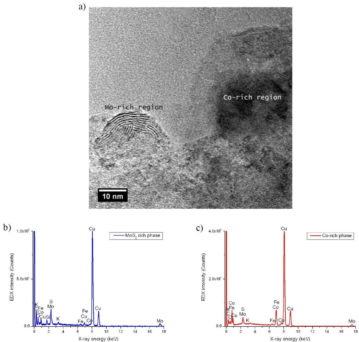
**Figure 2.** a) Image of a K promoted Co/MoS<sub>2</sub> catalyst for higher alcohol synthesis after *in situ* reduction in 1.5mbar  $\text{H}_2$  atmosphere at 630K. The phases were identified with EELS during the reduction and EDX post reduction. Figure 2b) shows the EDX scan on the Mo rich region and Figure 2c) the scan of the Co rich region, indicating the segregation.
