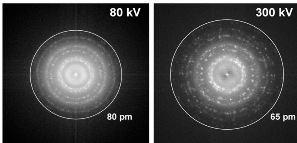
FIG. 1. Fourier transforms of  $C_C$  and  $C_S$  corrected HRTEM images of Au particles on a C support. The smallest detected image spacing at 80 kV (left) is  $\sim 80$  pm and at 300 kV (right) is  $\sim 65$  pm.
