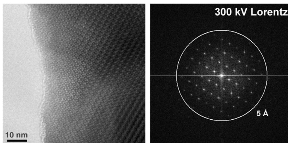
FIG. 3. Left:  $C_C$  and  $C_S$  corrected image of Cs<sub>0.5</sub>[Nb<sub>2.5</sub>W<sub>2.5</sub>O<sub>14</sub>] [001] acquired at 300 kV in Lorentz mode with the objective lens turned off. Right: Fourier transform revealing 5 Å image detail.
