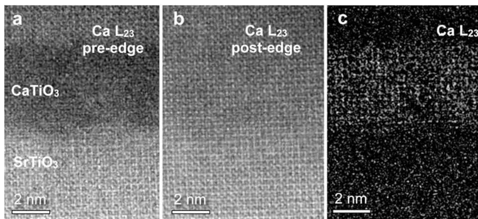
FIG. 2. Atomic resolution  $C_C$  and  $C_S$  corrected (a) Ca L<sub>23</sub> pre-edge and (b) Ca L<sub>23</sub> post-edge energy-loss images of a CaTiO<sub>3</sub>/SrTiO<sub>3</sub> [001] multilayer acquired at 300 kV using 10 eV energy-selecting windows and no objective aperture. (c) Background subtracted Ca map showing Ca on the A sites of the pseudo-cubic perovskite lattice.
