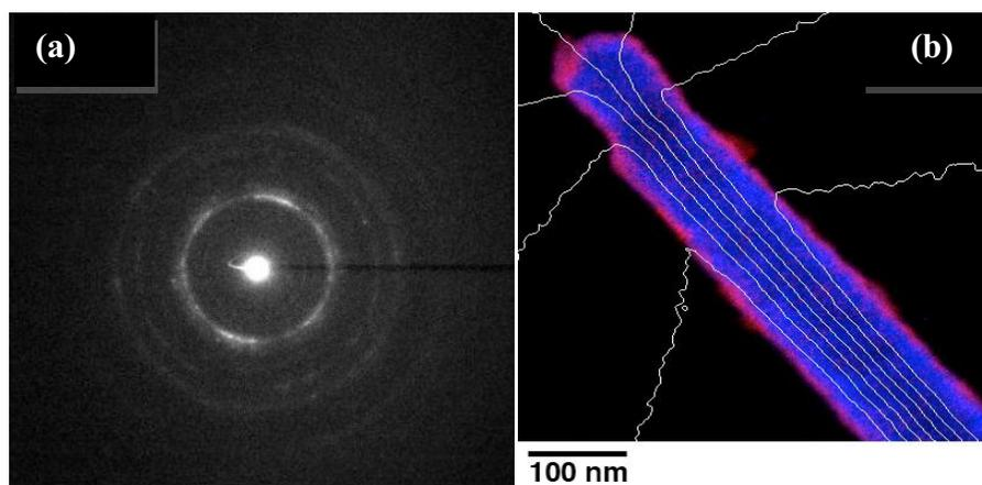
Fig. 1. (a) Electron diffraction pattern of a CoFeB wire, the d-spacings of the ring pattern are 1: 0.21 nm, 2: 0.13 nm and 3: 0.11 nm. (b) Magnetic contour image of a 170 nm diameter wire overlaid on an elemental map for Co (blue) and O (red). The contour spacing is 2 radians.
