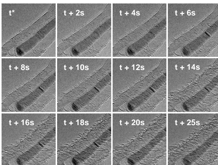
**Figure 3.** Sequence of bright-field TEM images showing the degradation of the CNT structure during exposure to the electron beam. \*the first micrograph was taken after several seconds (n.d.) of exposure to the electron beam.
