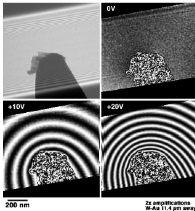
**Figure 1.** (a) Off-axis electron hologram of an unbiased tungsten tip acquired at 300 kV. (b-d) Reconstructed 2x amplified phase images for applied bias values of 0, 10 and 20 V, respectively, between the tip and a gold counter-electrode located  $\sim 10 \mu\text{m}$  away.
