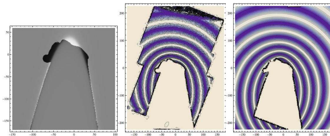
**Figure 2.** Left: Best-fitting tip shape parameters describing the major and minor semi-axes of the ellipsoidal null equipotential. Middle: Experimental 2x amplified phase image reconstructed from a hologram acquired with a 10 V applied bias. Right: Corresponding best-fitting simulated phase image, with the experimental tip outline superimposed.
