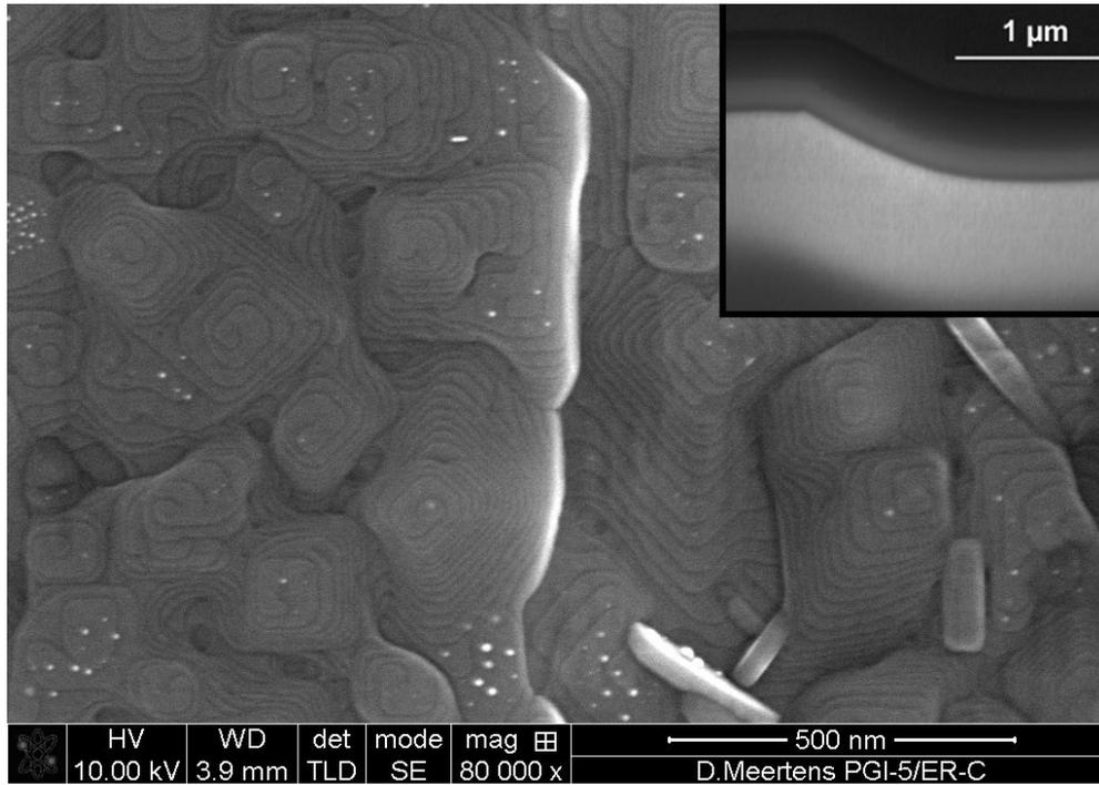
**Figure 1.** SEM image of the surface of a YBCO film deposited on an MgO substrate step edge. The inset in the top right corner shows a cross-section of a similar substrate edge structure made by FIB milling.
