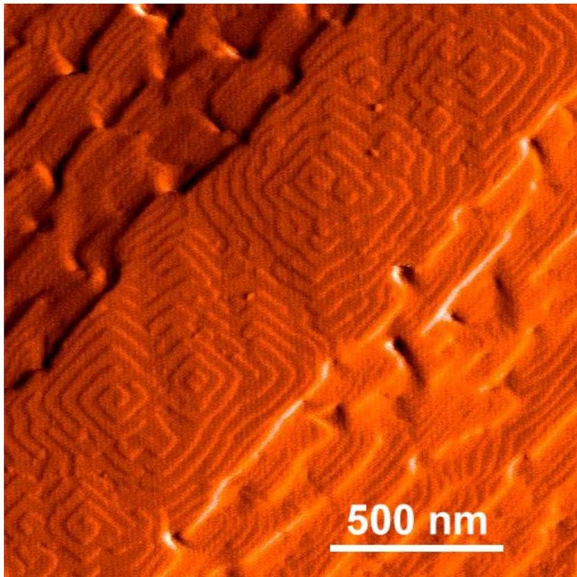
**Figure 2.** AFM image of a 140 nm thick YBCO film deposited on an IBE-cleaned trapezoidal feature on a (100) MgO substrate with 3 degree slopes on either side of the ridge.
