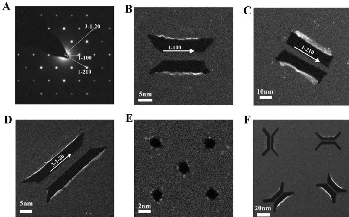
**Figure 1** (A) Diffraction of monolayer graphene (B-C) nano-ribbon along  $\langle 1-100 \rangle$ ,  $\langle 1-210 \rangle$ ,  $\langle 3-1-20 \rangle$  orientation respectively. (E) Pattern of nanopores with 2nm diameter (F) Pattern of nanoribbon with 1.2nm width, created using computer scripts.
