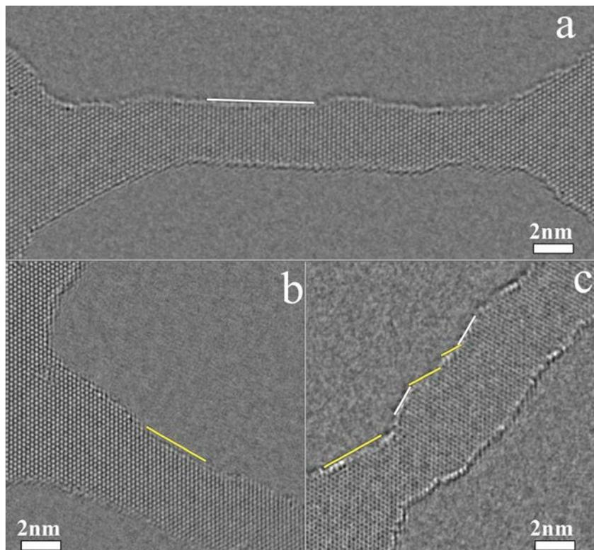
**Figure 2** (A-C) HREM images of nano-ribbons along  $\langle 1-100 \rangle$ ,  $\langle 1-210 \rangle$ ,  $\langle 3-1-20 \rangle$  respectively, recorded at 80kV using FEI Titan 60-300 PICO TEM, equipped with Cs-Cc achro-aplanat image corrector.
