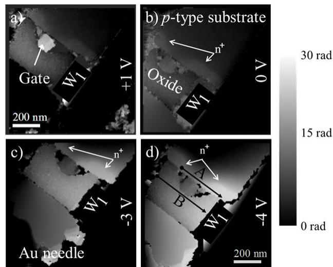
Figure 2) Phase images acquired from transistor  $T_1$  (marked in Fig.1a) under different biasing conditions. The  $pn$  junction between the  $n^+$  drain region under the  $W_1$  plug at the corner of the specimen and the  $p$ -type substrate was electrically biased, from 1V forward bias in a) to 4V reverse bias in d).
