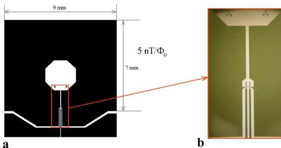
**Figure 2.** (a) Sketch of a direct coupled high- $T_c$  DC SQUID magnetometer with an 8 mm pick-up loop and step edge Josephson junctions. (b) Photograph of the inner part of the magnetometer with two DC SQUIDs. Each SQUID has an inductance of approximately 100 pH.
