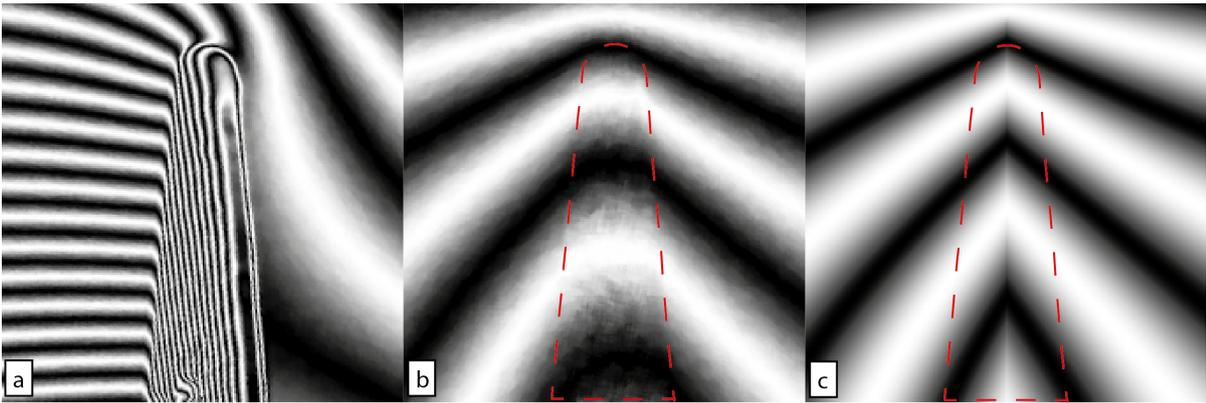
Fig. 1: Equiphase contours corresponding to a) an original phase image recorded from the needle; b) the difference between phase images acquired at two different bias voltages; c) a best-fitting model-dependent simulation to the result shown in b).
