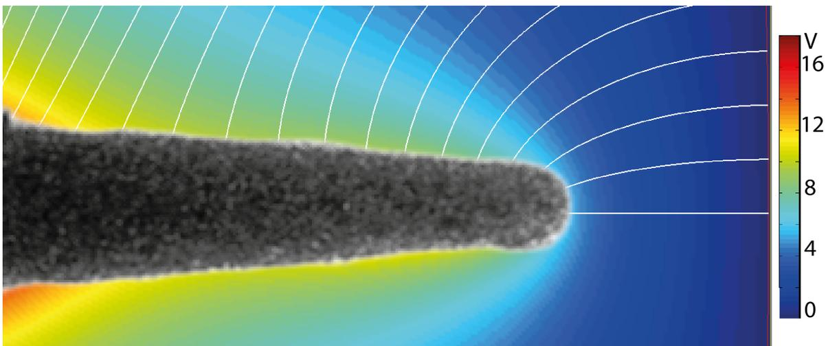
Fig. 3: Central slice of the three-dimensional distribution of electrical potential (colours) and electric field (white lines) around the needle, inferred from the results shown in Fig. 2.
