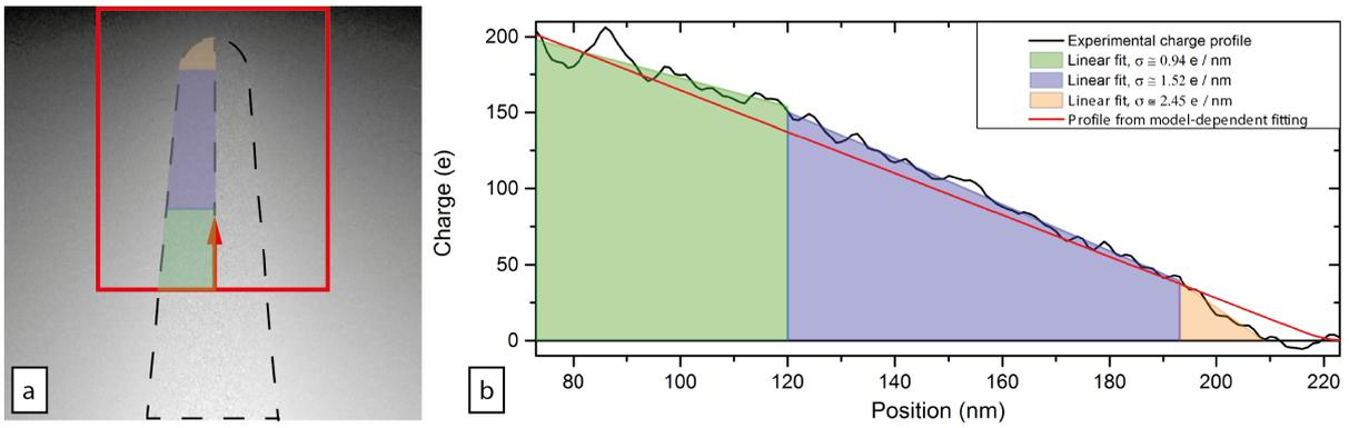
Fig. 2: a) Illustration of the use of an integration contour in the model-independent approach. b) Cumulative charge profiles measured using the model-independent (black) and model-dependent (red) methods.
