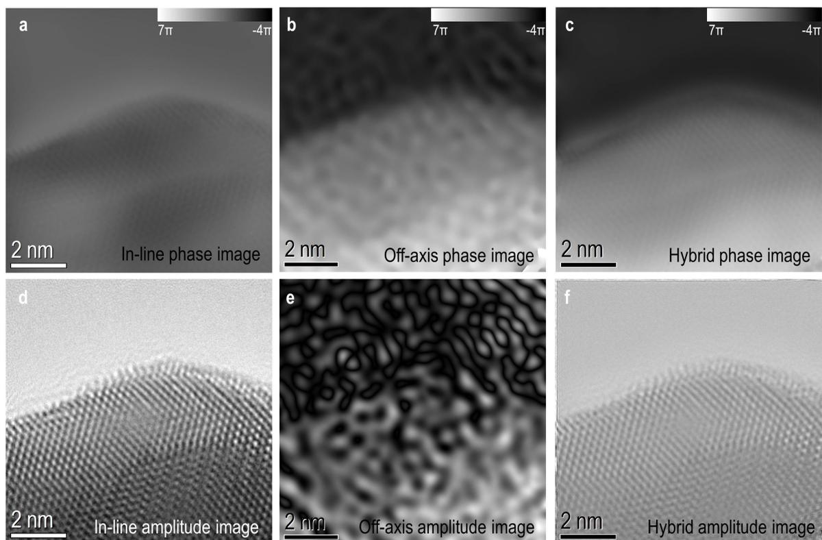
Fig. 1: a)-c) Reconstructed phase, d-f) reconstructed amplitude images from inline, off-axis and hybrid methods, respectively.
