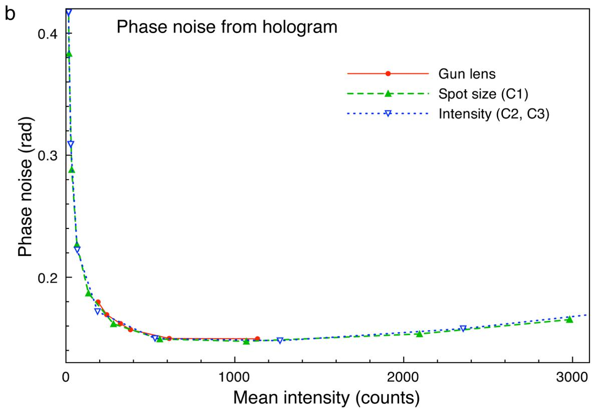
Fig. 1: (a) Hologram fringe contrast  $(I_{\max}-I_{\min})/(I_{\max}+I_{\min})$  and (b) standard deviation phase noise plotted against mean intensity within the overlap region for different settings of the gun lens, spot size and intensity.
