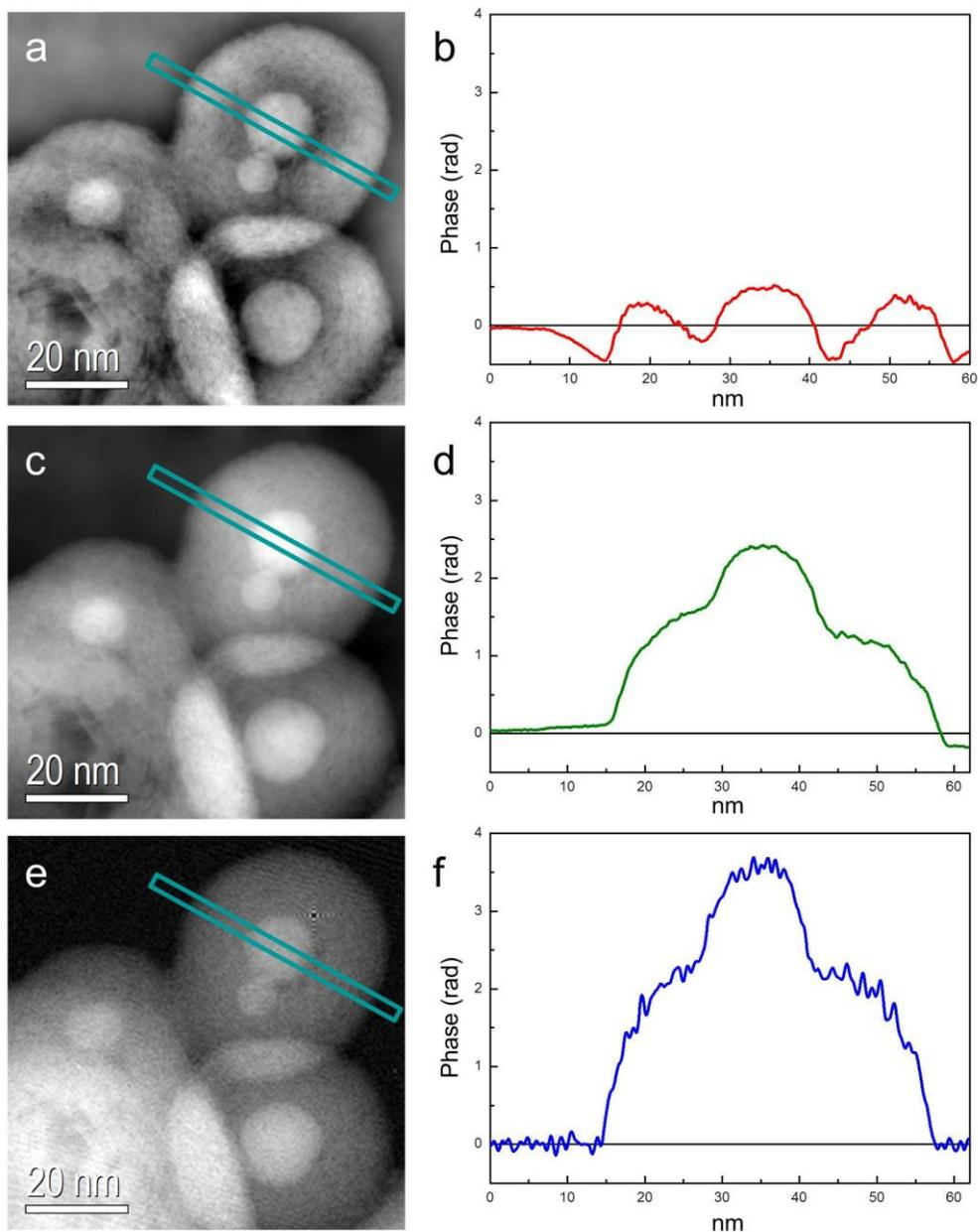
**Figure 1.** (a, c, e) Phase images and (b, d, f) corresponding line profiles across a feature within them. (a, b) Phase retrieved using conventional focal series reconstruction<sup>5</sup>. (c, d) Phase retrieved using gradient-flipping-assisted focal series reconstruction. (e, f) Phase retrieved using off-axis electron holography.
