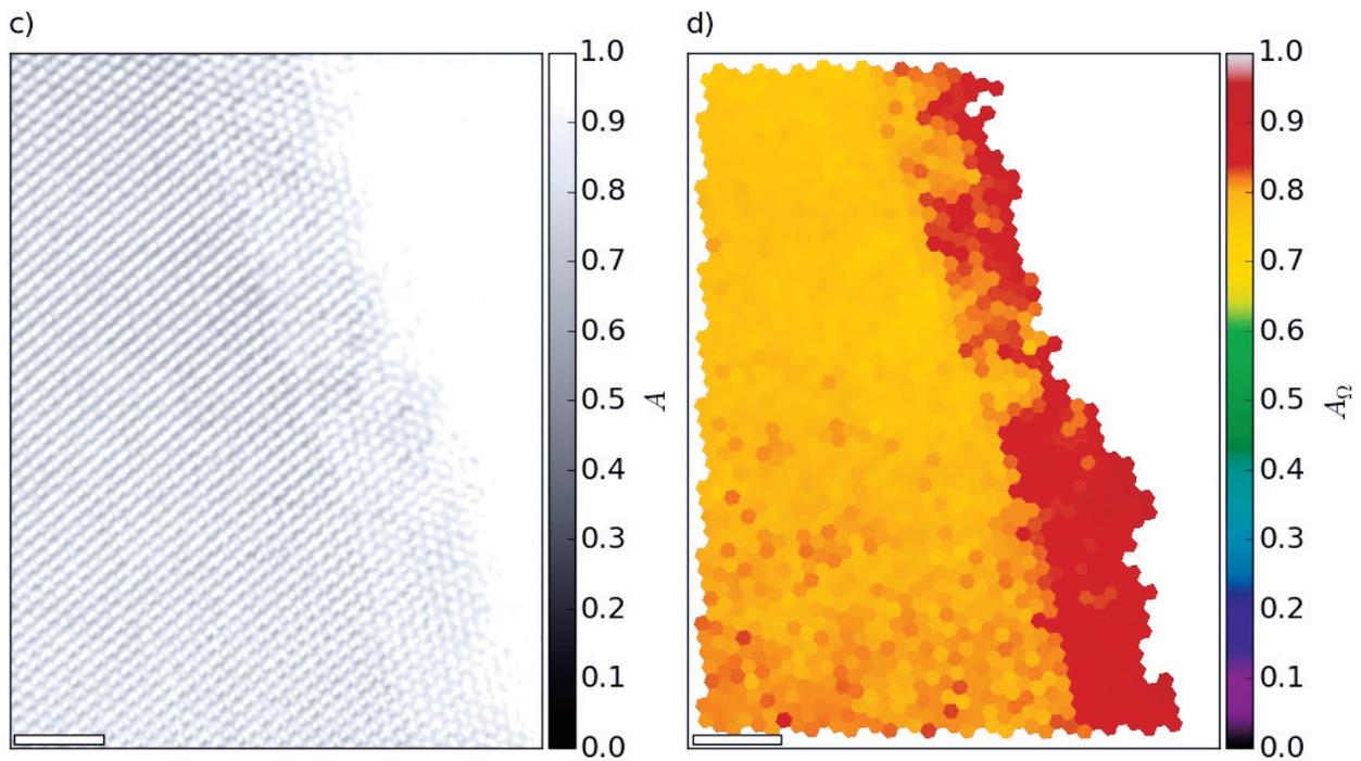
a) Phase  $\Phi$  and b) amplitude  $A$  images of a few-layer-thick WSe<sub>2</sub> flake with a vacuum area at the right side and a thinner, but also contaminated region close to the edge of the specimen. c)  $\Phi$  and d)  $A$  after averaging within the area of each Voronoi cell  $\Omega$  constructed from the phase image in a). The scale bars are 2 nm.
