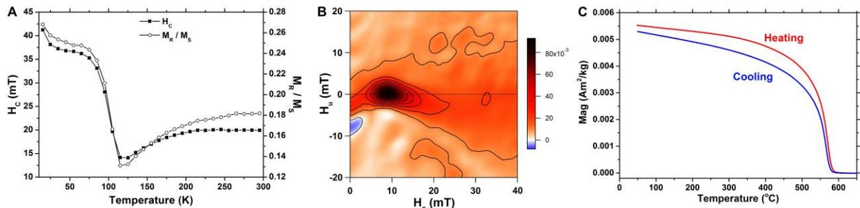
**Figure 2.** (A) Graph of coercive force and  $M_{rs}/M_s$  as a function of temperature (15 K to 295 K). (B) FORC diagram acquired at room temperature (smoothing factor = 7). The measurement time was 250 ms. (C) Thermomagnetic curves of the synthetic basalt. Heating was performed in flowing helium, in a field of 300 mT.
