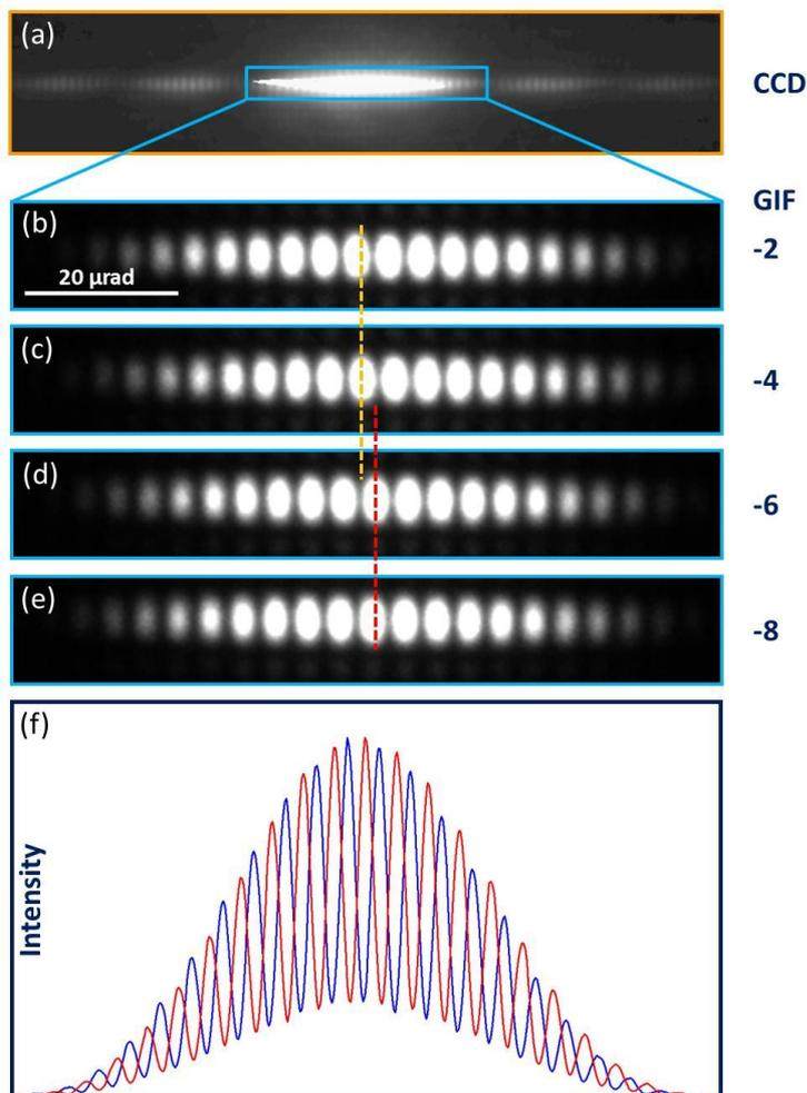
**Figure 2.** (a) Low-angle electron diffraction image recorded using a conventional charge-coupled device (CCD) camera located before the Gatan imaging filter (GIF). (b)–(e) Low-angle electron diffraction images recorded using the GIF CCD camera after tilting the sample between  $-2^\circ$  and  $-8^\circ$  in steps of  $-2^\circ$ . (f) Line scans of (c) in blue and (d) in red.
