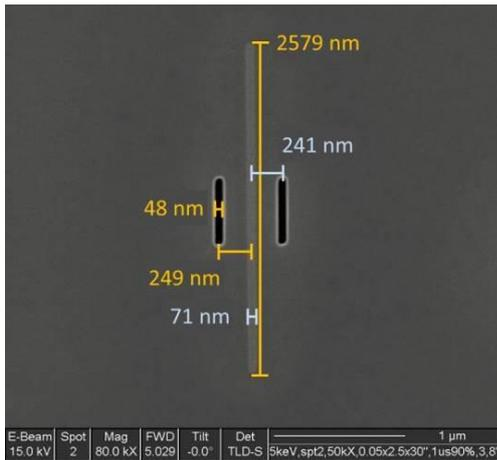
**Figure 1.** Secondary electron image of the two slits and the Co nanorod. The slits are the dark features on either side of the Co nanorod.
