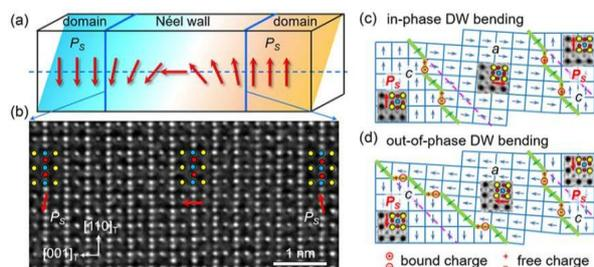
**Figure 1.** (a) Schematic representation of a Néel-type DW. (b) The Néel-like DW imaged in  $x = 0.60$  PZT crystal. (c) The in-phase and (d) out-of-phase bent ferroelastic DWs in the  $x = 0.9$  PZT thin films.
