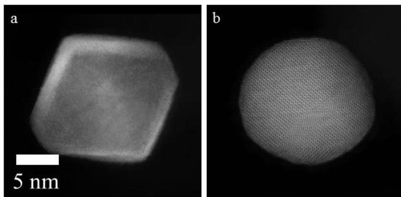
**Figure 1.** HAADF-STEM images of (a) an octahedral PtNi NP with a segregated structure under reducing conditions at 300 °C; (b) the same NP shapeless after examination at 600 °C under reducing conditions.
