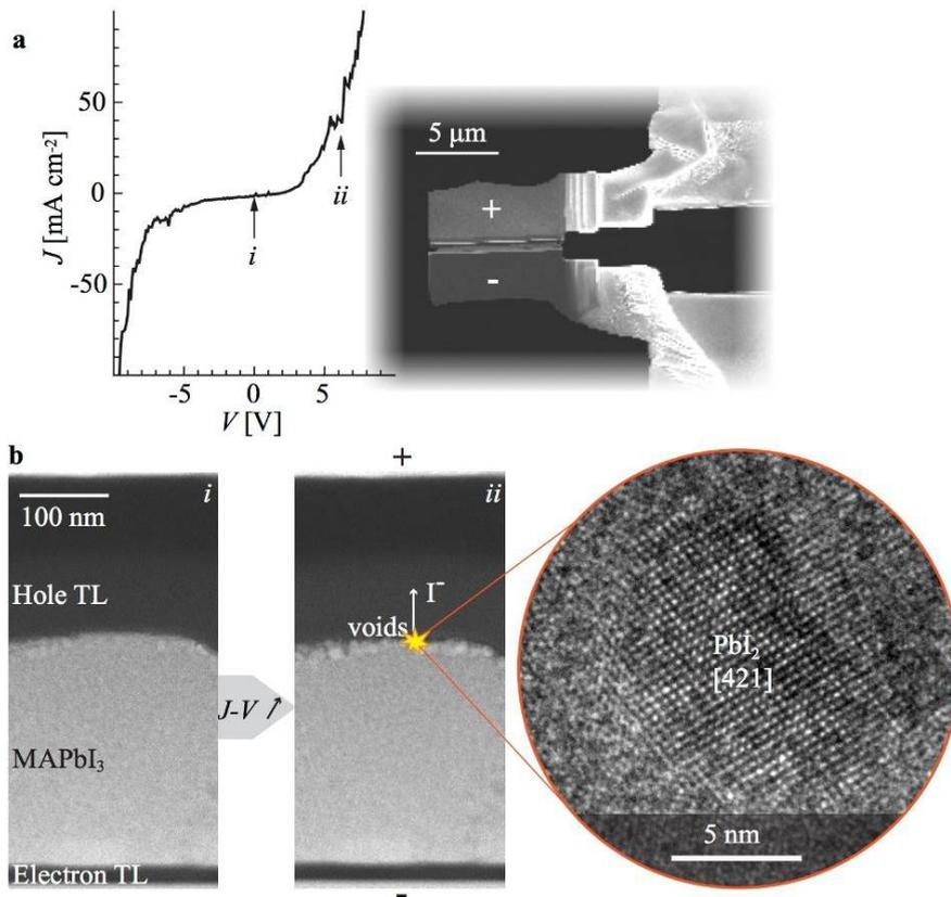
**Figure 1.** (a)  $J$ - $V$  curve recorded *in situ* in the TEM alongside the MEMS-contacted TEM lamella. (b) STEM high-angle annular dark-field images recorded (i) before and (ii) after applying a bias of 6 V to the sample, resulting in  $\sim 50$  mA cm $^{-2}$  passing through it, the migration of iodide towards the positively biased electrode and the formation of voids and PbI $_2$  at the interface with the hole transport layer (TL).
