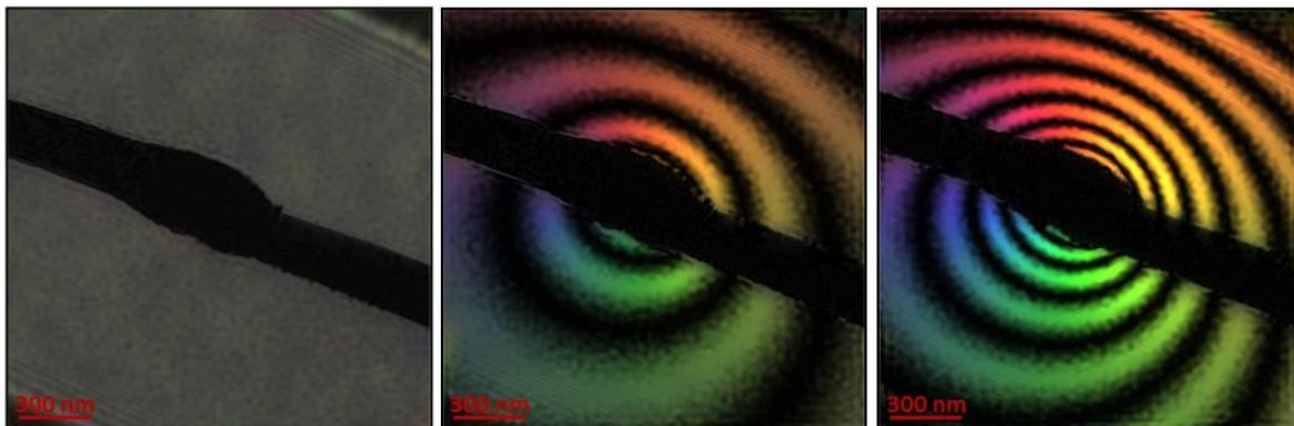
**Figure 2.** 8x amplified phase images of the vacuum region around the contacted TAPP recorded using off-axis electron holography for currents of 0 (left), 2 mA (middle) and 4 mA (right).
