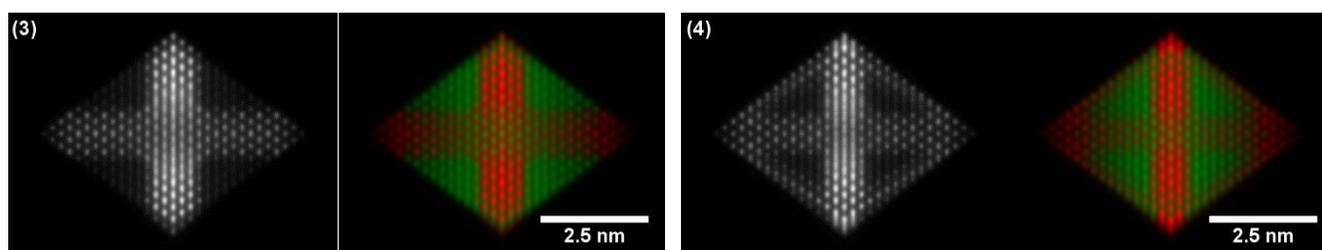
**Figure 1.** Two example simulated structures showing both the ADF STEM image and the EDX map close to a  $\langle 110 \rangle$  orientation for Pt hexapod (3) and Pt hexapod and edges (4). The Pt-L line is shown in red, the Ni-K is in green.
