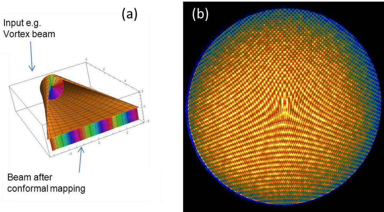
Fig 1 a) Schematic diagram illustrating conformal mapping by a Fan-out OAM sorter. b) Main hologram of a Fan-out sorter.
