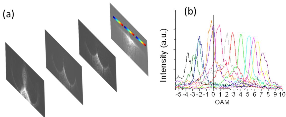
Fig.2 a) Beam evolution in a sorter. b) Experimental OAM spectra for various vortex beams
