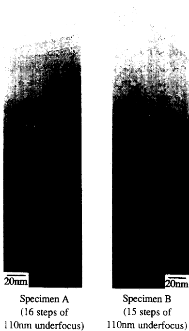
Fig. 1. TEM images taken from through-focal series of specimens A and B, at the defocus values indicated. The positions of the regions which were extracted digitally for analysis, and which correspond to intensities of 0.7, 0.6 and 0.55 relative to the value of 1 at zero crystal thickness in each specimen, are marked using the symbols 1, 2 and 3, respectively.
