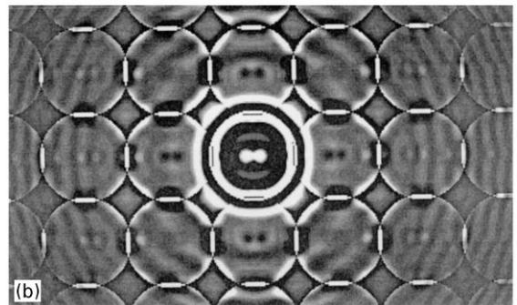
Fig. 6. (a) Simplified diagram for the STEM crystal-focuser case. (b) Image formed for a specimen consisting of two Au atoms,  $0.68 \text{ \AA}$  apart, illuminated by a STEM beam ( $200 \text{ keV}$ ,  $C_s = 1 \text{ mm}$ ) and placed at the Fourier image distance of  $332 \text{ \AA}$  from an Au  $[001]$  crystal,  $2.8 \text{ nm}$  thick.
