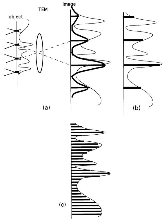
Fig. 4. (a) Diagram illustrating the crystal-focuser TEM scheme. The specimen is illuminated by the array of very fine cross overs and for each cross over the TEM gives an image of normal TEM resolution on the image plane. For each peak a corresponding intensity value is assigned to the peak-center position as in (b). The sets of values found for all incident-beam tilts are correlated to form the ultra-high-resolution image (c).
