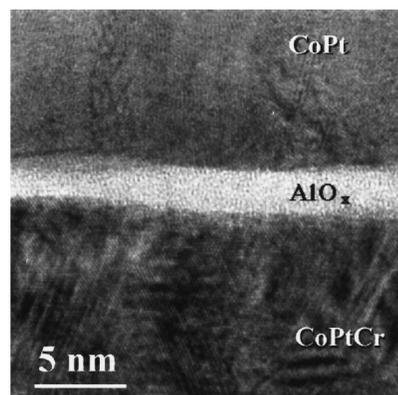
FIG. 1. Representative cross-sectional image of CoPtCr/AlO<sub>x</sub>/CoPt tunnel junction, as deposited.
