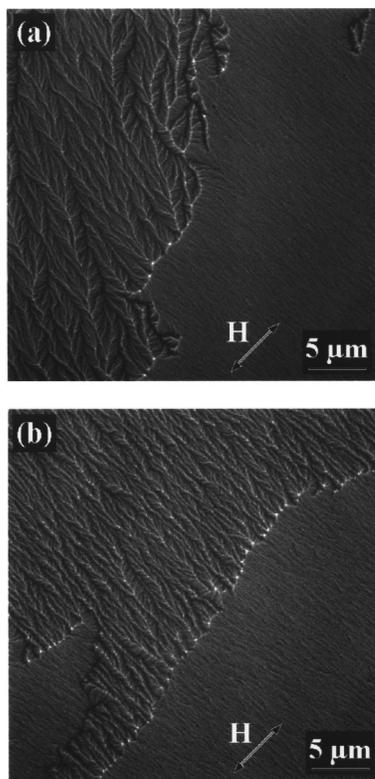
FIG. 3. Lorentz images at coercive field during magnetization reversal of: (a) 15 nm Co soft layer and (b) 15 nm Ni<sub>40</sub>Fe<sub>60</sub> soft layer, with underlying 10 nm CoPtCr layer fully magnetized in the direction of the arrow.
