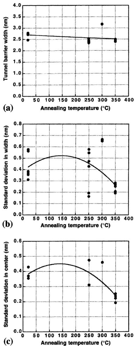
FIG. 2. Characteristics of alumina tunnel barrier as function of annealing temperature as measured from high-resolution images: (a) tunnel barrier width; (b) the standard deviation in this mean width; and (c) the standard deviation in the position of the center of the layer.
