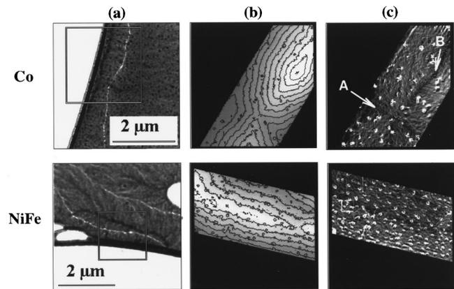
FIG. 4. (a) Lorentz images of domain walls in soft layers alone supported on holey carbon film. (b) Contours superimposed on electron holographic phase image of areas marked in (a). (c) Magnitude of in-plane component of magnetic induction integrated in incident beam direction. Features of interest are dark lines at positions of domain walls, which provide evidence for presence of asymmetric Néel walls. (Small white circles are surface oxide particles; their contrast is not magnetic.)
