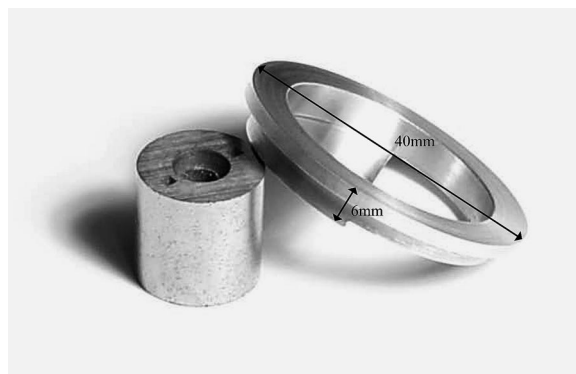
Fig. 1. The aluminium insert and knife edge used to measure the MTF of the 1k^2 CCD camera.
