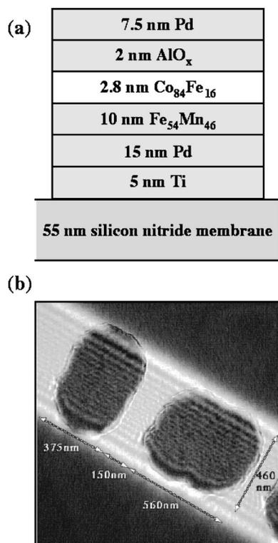
FIG. 1. (a) Schematic diagram showing nominal layer thicknesses in exchange-biased patterned elements; (b) Off-axis electron hologram of two rectangular elements showing typical lateral dimensions.
