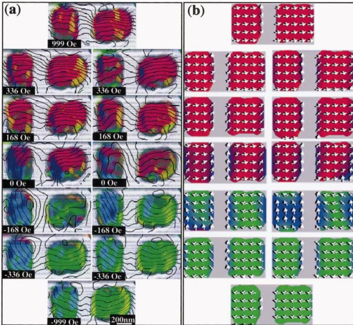
FIG. 2. (Color) Comparison of (a) experimental holographic phase measurements and (b) micromagnetic simulations during complete magnetization reversal cycle for exchange-biased  $\text{Co}_{84}\text{Fe}_{16}/\text{Fe}_{54}\text{Mn}_{46}$  patterned elements. Applied in-plane fields, which are directed along the horizontal axis, are shown at the bottom left corner of each phase image. Colors represent different magnetization directions. Phase contours are separated by  $0.085\pi$  radians.
