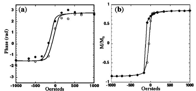
FIG. 3. Hysteresis loops for larger exchange-biased element: (a) measured from experimental holograms; (b) derived from micromagnetic simulations.
