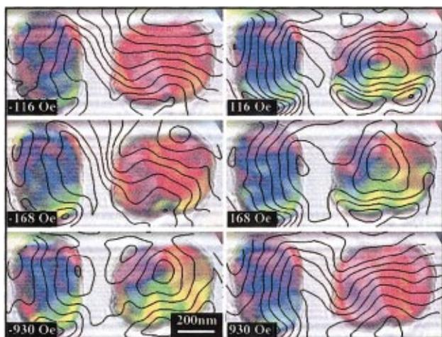
FIG. 4. (Color) Remanent states for exchange-biased elements. Left-hand set obtained after saturation of elements to the right followed by reversal to the value indicated. Similarly for the right-hand set except initial saturation direction to the left.
