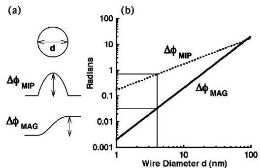
FIG. 1. (a) Schematic diagrams showing the MIP and magnetic (MAG) contributions to the phase shift of an electron wave that traverses a magnetic nanowire of diameter  $d$ . (b) Graph showing  $\Delta\phi_{\text{MIP}}$  (dotted line) and  $\Delta\phi_{\text{MAG}}$  (solid line) for a Co nanowire, plotted as a function of wire diameter.
