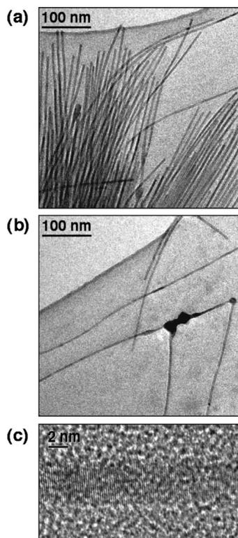
FIG. 2. Bright-field TEM images of (a) the end of a bundle of Co nanowires adjacent to a hole in the C support film, (b) a multibranch nanowire, comprising several nanowires joined together at junctions, and (c) [0002] Co lattice fringes visible along the length of an isolated wire.
