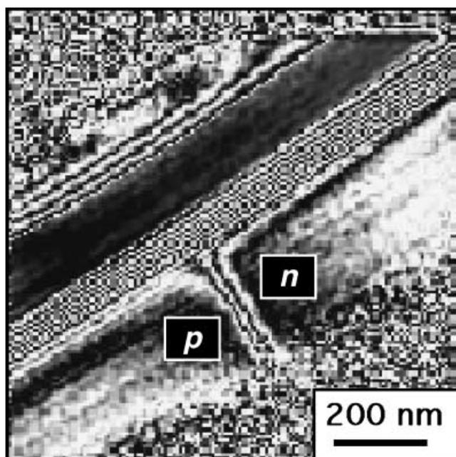
Fig. 14. Four-times-amplified cosine of the measured phase acquired from a focused ion beam milled specimen at a reverse bias voltage of 3 V, reconstructed using the zero volt bias image as a reference hologram. Note the absence of electrostatic fringing fields in the vacuum region outside the specimen edge.
