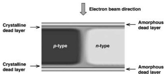
Fig. 13. Schematic diagram showing, in cross-section, the physical and electrical structure of a focused ion beam milled TEM specimen inferred from the present study.
