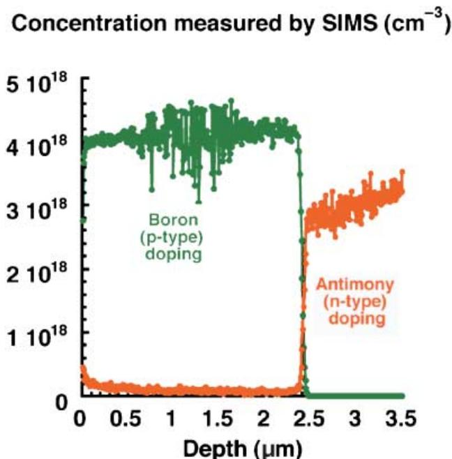
Fig. 2. Secondary ion mass spectrometry (SIMS) profile obtained from the sample examined in this study, which contains a single  $p$ - $n$  junction at a depth of 2.5  $\mu\text{m}$  below the wafer surface.
