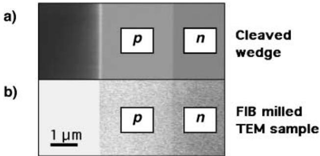
Fig. 15. Scanning electron microscope (SEM) images acquired by collecting secondary electrons from (a) a 90° cleaved wedge, and (b) a focused ion beam milled TEM membrane containing the Si  $p$ - $n$  junction examined in this study.
