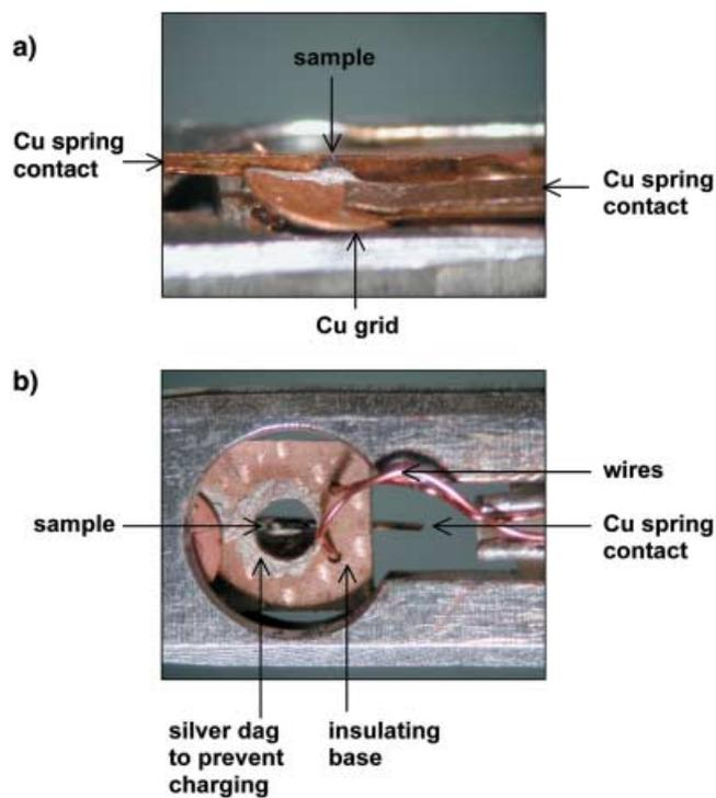
Fig. 6. Annotated photographs showing a *p-n* junction specimen in the biasing holder, viewed from (a) above and (b) below. The semicircular Cu grid shown in (a) has a diameter of 3 mm.
