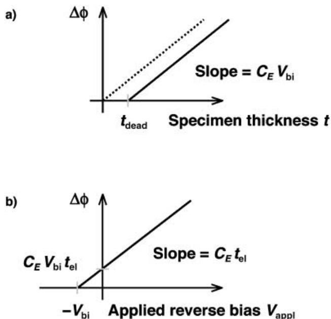
Fig. 9. Schematic diagrams showing graphs of the step in phase  $\Delta\phi$  across a  $p$ - $n$  junction expected as a function of (a) the total specimen thickness, and (b) the reverse bias applied across the TEM specimen.
