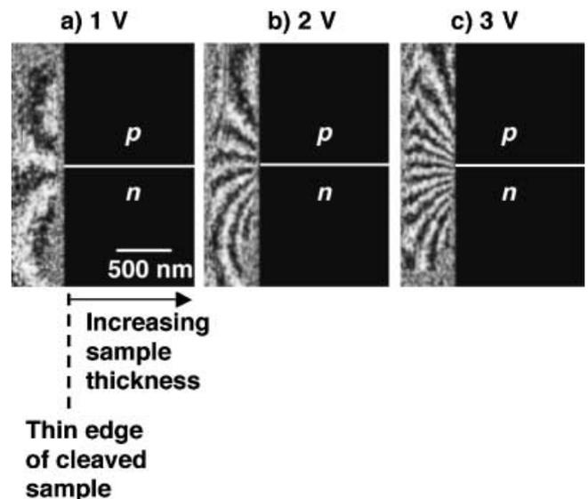
Fig. 7. Four-times-amplified cosine of the measured phase, showing the electrostatic fringing field in the vacuum region outside the position of the *p-n* junction in a  $90^\circ$  cleaved wedge that had not been FIB milled, for the three different applied reverse bias voltages indicated. The zero bias hologram was used as the reference hologram when forming each phase image. The phase shift inside the present specimen, whose thickness increases rapidly, could not be reconstructed successfully.
