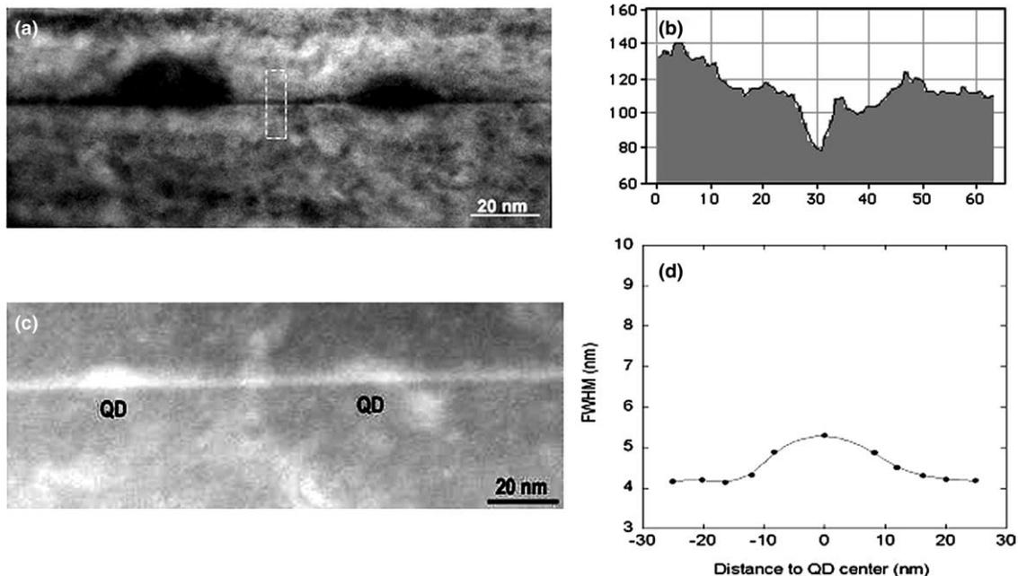
Fig. 4. (a) TEM bright field image of InAs QD buried in GaAs matrix, (b) intensity profile from the marked region showing the wetting layer in the image (a), (c) HAADF image of small coherent InAs QD in GaAs matrix, and (d) EDX peak width (FWHM) at different lateral position of a buried QD.
