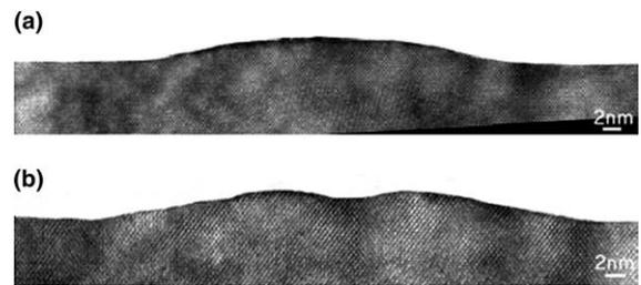
Fig. 2. [1 1 0] Zone cross-sectional HRTEM images of, (a) an isolated QD, and (b) two neighbouring QDs after 5 Å GaAs capping.
