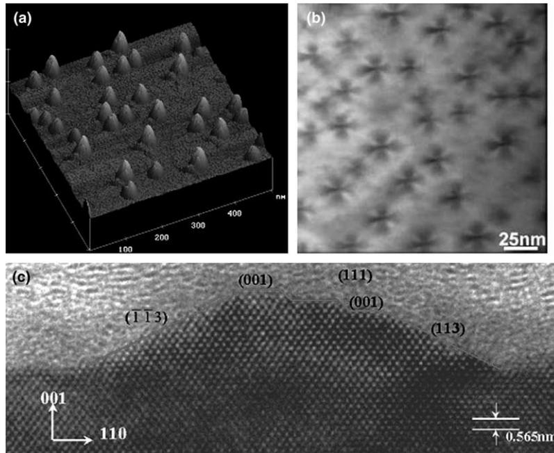
Fig. 1. (a) AFM image of uncapped QDs, (b) [00 1] zone plan-view BF TEM image of unburied QDs, and (c) [1  $\bar{1}$  0] zone HRTEM image of uncapped QDs.
