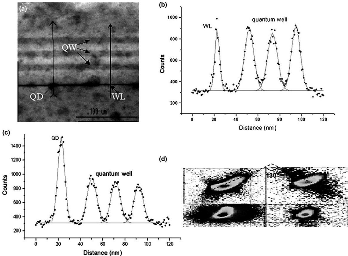
Fig. 5. (a) STEM image from a QD sample containing three  $\text{In}_{0.12}\text{Ga}_{0.88}\text{As}$  QWs, (b) and (c) show EDX line-scan profiles through wetting layer and QD, respectively, (d) 400, 040, 220 and  $-220$  experimental reciprocal space maps from in-plane X-ray scattering.
