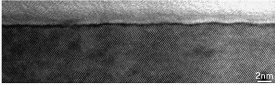
Fig. 3. Cross-sectional HRTEM image of QD after 15 Å GaAs capping.
