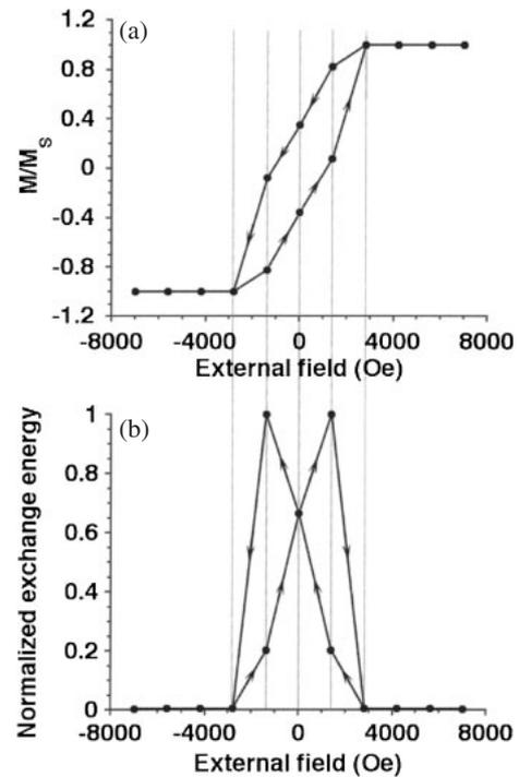
**Fig. 8.** Representative results from micromagnetic simulations showing (a) a hysteresis loop and (b) the variation in exchange energy in a chain of three spheres during magnetization reversal. The calculation was carried out for a chain of Fe spheres, with a central sphere diameter  $d_c$  of 50 nm and outer sphere diameters  $d_o$  of 75 nm.
