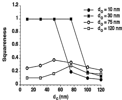
**Fig. 13.** Values of squaresness ( $M_R/M_S$ ) calculated for chains of three spheres of  $Fe_{20}Ni_{80}$ , plotted as a function of central sphere diameter  $d_c$  for a range of outer sphere diameters  $d_o$ .
