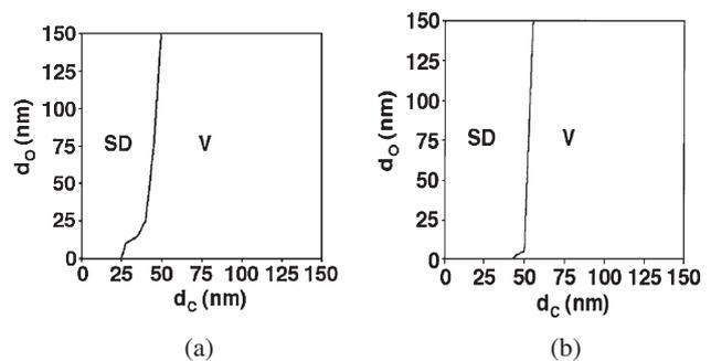
**Fig. 3.** Results of micromagnetic simulations, showing the magnetic remanent states that form in the central sphere in a chain of three spheres of (a) Fe and (b) Ni, plotted as a function of both the central sphere diameter  $d_c$  and the outer sphere diameters  $d_o$ . SD and V refer to single domain and vortex states, respectively.
