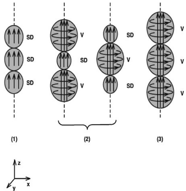
**Fig. 2.** Schematic diagrams showing the different magnetic remanent states observed in the linear chains of three spheres using micromagnetic simulations. SD and V refer to single domain and vortex states, respectively. The chain axes lie parallel to the z axis.
