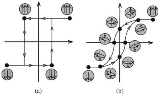
**Fig. 4.** Schematic diagrams, based on the results of micromagnetic simulations, showing the evolution of magnetic states during magnetization reversal in (a) isolated spheres that contain single domains and (b) isolated spheres that are large enough to support vortices. The external field is applied in the vertical direction (along the z axis).
