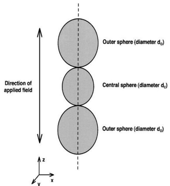
Fig. 1. Geometry of the linear chain of three spheres. The central sphere has diameter  $d_c$ , the outer spheres have diameters  $d_o$ , and external fields are applied parallel to the chain axis. The chain axis lies parallel to the  $z$  axis.
