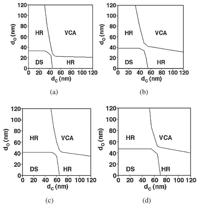
**Fig. 7.** Results of micromagnetic simulations showing the magnetization reversal mechanisms that are observed in chains of three spheres of (a) Fe, (b)  $Fe_{56}Ni_{44}$ , (c)  $Fe_{20}Ni_{80}$ , and (d) Ni, plotted as a function of both the central sphere diameter  $d_c$  and the outer sphere diameters  $d_o$ . DS, HR, and VCA refer to single domain switching, hybrid reversal and vortex creation and annihilation, respectively, as described in the form of schematic diagrams in Fig. 5.
