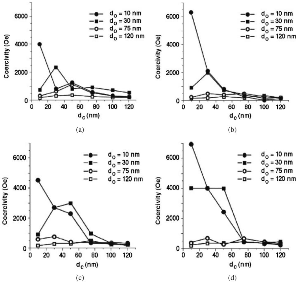
**Fig. 12.** Results of micromagnetic simulations showing the coercivities of chains of three spheres of (a) Fe, (b)  $Fe_{56}Ni_{44}$ , (c)  $Fe_{20}Ni_{80}$ , and (d) Ni, plotted as a function of central sphere diameter  $d_c$  for a range of outer sphere diameters  $d_o$ .
