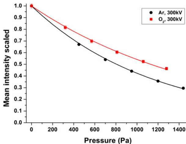
2 Normalised image intensity (without specimen present) measured on pre-GIF UltraScan CCD camera, plotted as function of gas pressure for Ar and O<sub>2</sub>. Primary electron energy is 300 keV. Data points have been fitted to exponential functions
