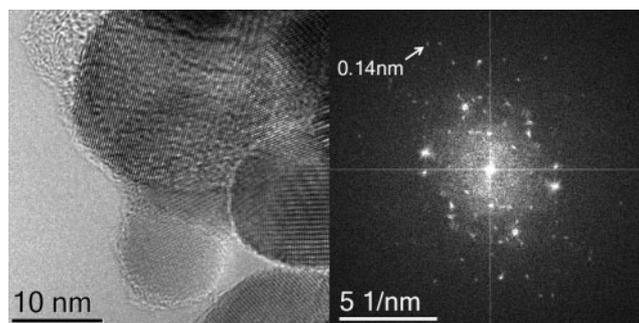
**5 High resolution lattice image of  $\text{ZrO}_2$  particles in 1:1 mixture of  $\text{H}_2$  and  $\text{N}_2$  recorded at total gas pressure of 310 Pa and at specimen temperature of 177°C: Fourier transform provides indication of stability of microscope and specimen under these conditions**
