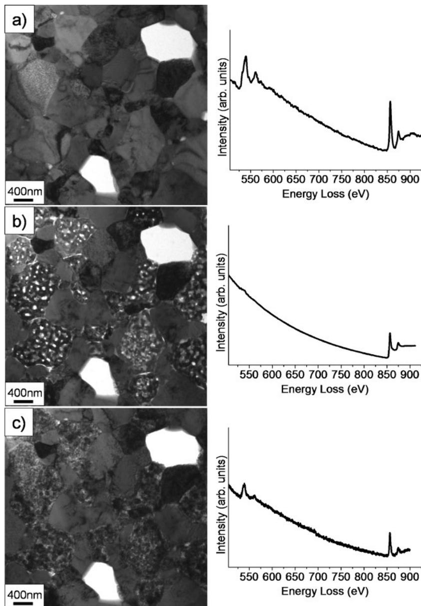
a before reduction at room temperature in normal TEM mode; b after *in situ* reduction in 130 Pa H<sub>2</sub> at 500°C for 2 h; c after *in situ* reoxidation in 320 Pa O<sub>2</sub> at 500°C for 2 h
