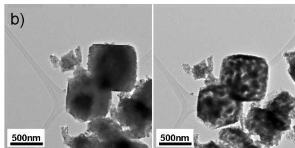
**a** low loss EELS of NiZn sample before (in high vacuum) and after (120 Pa  $\text{H}_2$ ,  $T=450^\circ\text{C}$ ) *in situ* reduction; **b** TEM images of corresponding as prepared (left) and reduced (right) samples
