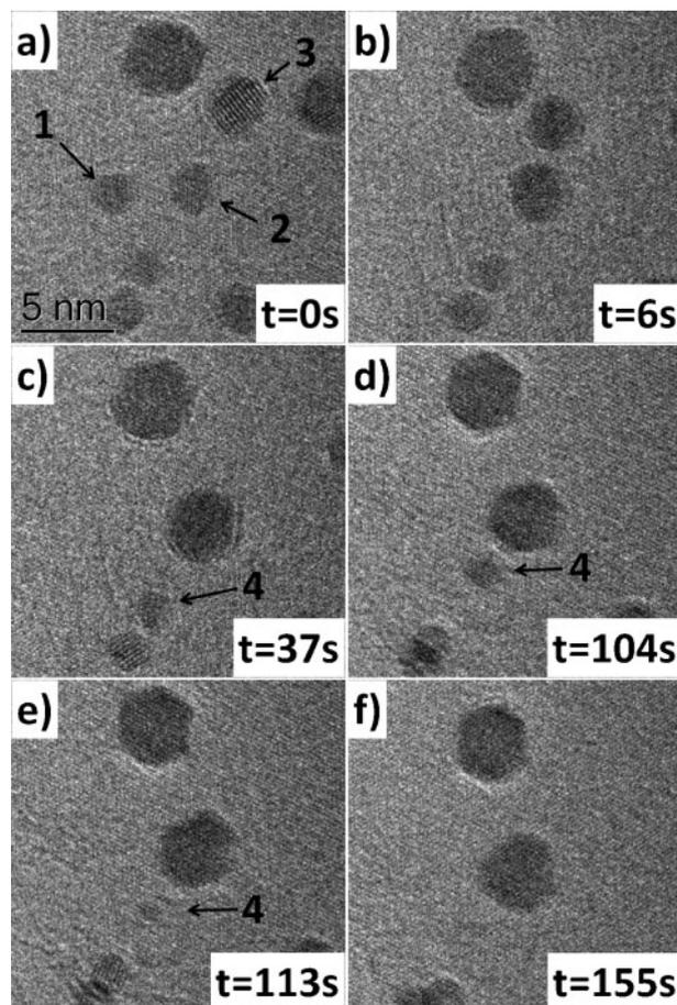
**4** Frames taken from sequence of bright field images of gold particles on boron nitride support imaged in 130 Pa of H<sub>2</sub> at 410°C: images were recorded using 300 kV primary electron beam with *C*<sub>s</sub> set to below 5 μm (see text for more details)
