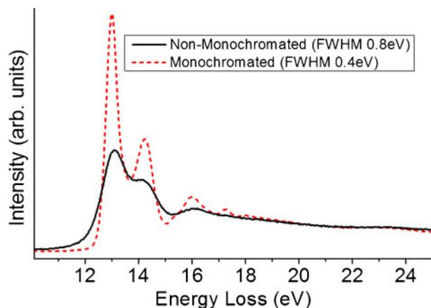
7 Non-monochromated and monochromated EELS of N<sub>2</sub> gas acquired *in situ* at 500 Pa at room temperature
