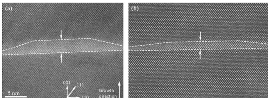
Fig. 1. High-resolution Z-contrast HAADF STEM images of (a) Sample A and (b) sample B in cross-sectional geometry. The dotted lines mark the outline of the QDs and the arrows denote the measured height of them. Both specimens are oriented along the  $[\bar{1} 1 0]$  zone-axis.
