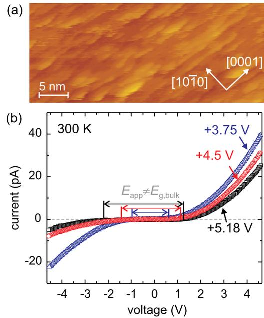
FIG. 2. (a) Constant-current empty state STM image of a stepped ZnO(11 $\bar{2}$ 0) cleavage surface measured at a voltage of  $V_{\text{set}} = +3.6$  V and current of  $I_{\text{set}} = 30$  pA. (b) Current-voltage curves (shown as symbols) acquired at the stepped ZnO(11 $\bar{2}$ 0) cleavage surface with different tip-sample separations, adjusted using different  $V_{\text{set}}$  as labeled.  $E_{\text{app}}$  indicates the voltage range without detectable tunnel current.
