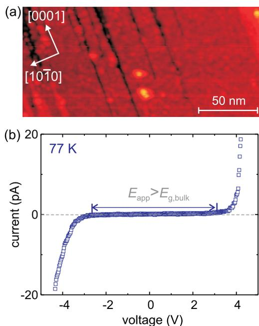
FIG. 1. (a) Constant-current empty state STM image of a ZnO(11 $\bar{2}$ 0) cleavage surface with few monolayer high cleavage steps measured at a voltage of  $V_{\text{set}} = -5.0$  V and current of  $I_{\text{set}} = 10$  pA. (b) Current-voltage ( $I$ - $V$ ) curve acquired on the terrace far away from the steps.  $E_{\text{app}}$  indicates the voltage range without detectable tunnel current, called *apparent* bandgap.
