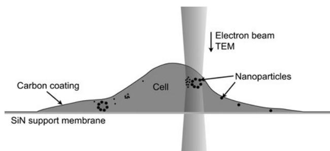
**Figure 1.** Schematic diagram depicting transmission electron microscopy (TEM) of a whole mount cell. The cell was grown on a silicon nitride (SiN) support membrane, fixed and critical point dried. A thin coating of carbon increased the stability of the cell under electron beam irradiation. Two different sizes of gold nanoparticles were used as specific protein labels to study the uptake processes of low-density lipoprotein.
