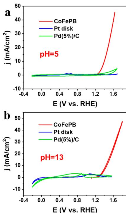
**Figure 5.** Cyclic voltammograms ( $5 \text{ mV s}^{-1}$ ) with CoFePB, Pt, and Pd(5%)/C catalysts (a) pH 5 and (b) pH 13 aqueous solutions containing 0.4 M formate and 1 M  $\text{KNO}_3$ . CVs of the Pt and Pd catalysts can be observed in more detail in Figure S11.
