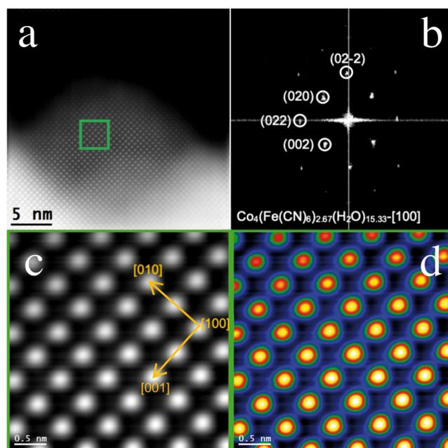
**Figure 1.** (a) Atomic resolution HAADF STEM image showing the edge of a nanocube. (b) Respective power spectrum (FFT) confirming that the nanocube structure is in agreement with the Co<sub>4</sub>(Fe(CN)<sub>6</sub>)<sub>2.67</sub>(H<sub>2</sub>O)<sub>15.33</sub> (FM3-M; space group, 225) crystal phase in the [100] direction. (c, d) Enlarged image from the green squared section in both gray and temperature colored scales.
