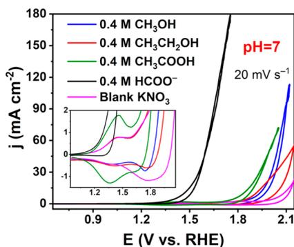
**Figure 4.** Cyclic voltammograms ( $20 \text{ mV s}^{-1}$ ) with a CoFePB working electrode in the presence of small organic molecules (formic acid, methanol, ethanol, and acetic acid) in  $1 \text{ M KNO}_3$  aqueous solution at pH 7.
