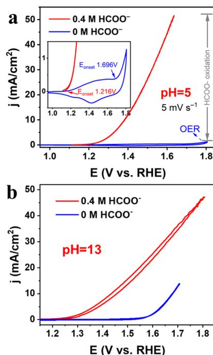
**Figure 2.** Cyclic voltammograms (CVs) on CoFePB electrodes in (a) pH 5 and (b) pH 13 aqueous solutions in the presence (red line) and absence (blue line) of 0.4 M HCOO<sup>-</sup>. Electrolyte, 1 M KNO<sub>3</sub>. Scan rate, 5 mV s<sup>-1</sup>. Note, oxidation waves that are typical of formate oxidation with Pt or Pd are not observed here because CoFePB has a different electrochemical mechanism, *vide infra*.
