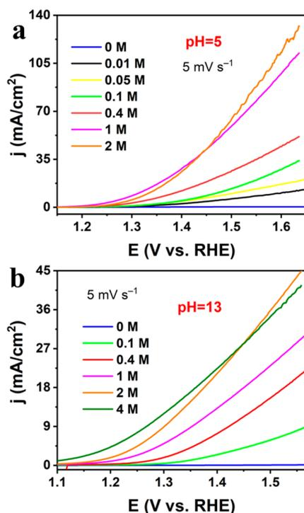
**Figure 3.** Anodic polarization data on CoFePB electrodes in 1 M KNO<sub>3</sub> aqueous electrolyte at 5 mV/s scan rates. Current density as a function of [HCOO<sup>-</sup>] at (a) pH 5 and (b) pH 13.
