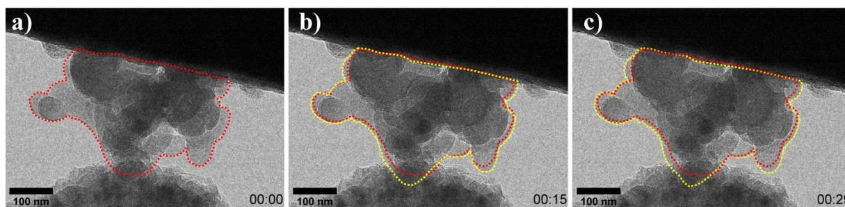
**Figure S6.** Chemical lithiation of a Si nanoparticle cluster. The red dotted line marks the shape of the cluster before chemical lithiation. The yellow dotted line shows the shape of the cluster at the indicated point in time during chemical lithiation.
