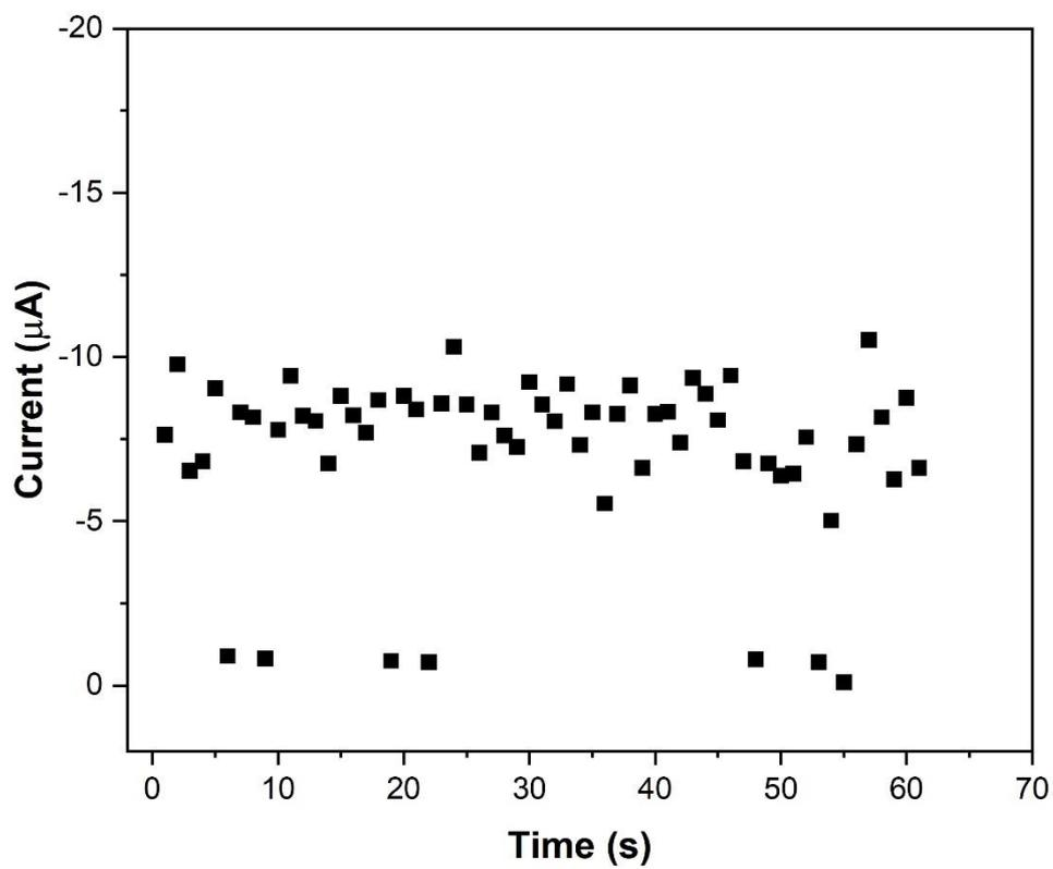
**Figure S4.** Current during the lithiation of the Si nanoparticle cluster shown in Figure 2 at  $-0.2V$ .
