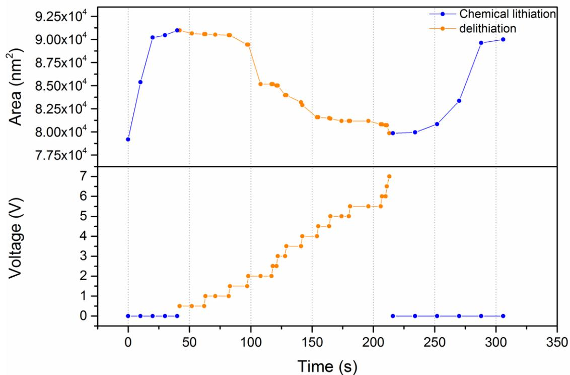
**Figure S7:** Expansion and contraction of a Si nanoparticle cluster during repeated (chemical) lithiation and delithiation. The plots show the area of the cluster measured from TEM micrographs and the corresponding bias voltage as a function of time.
