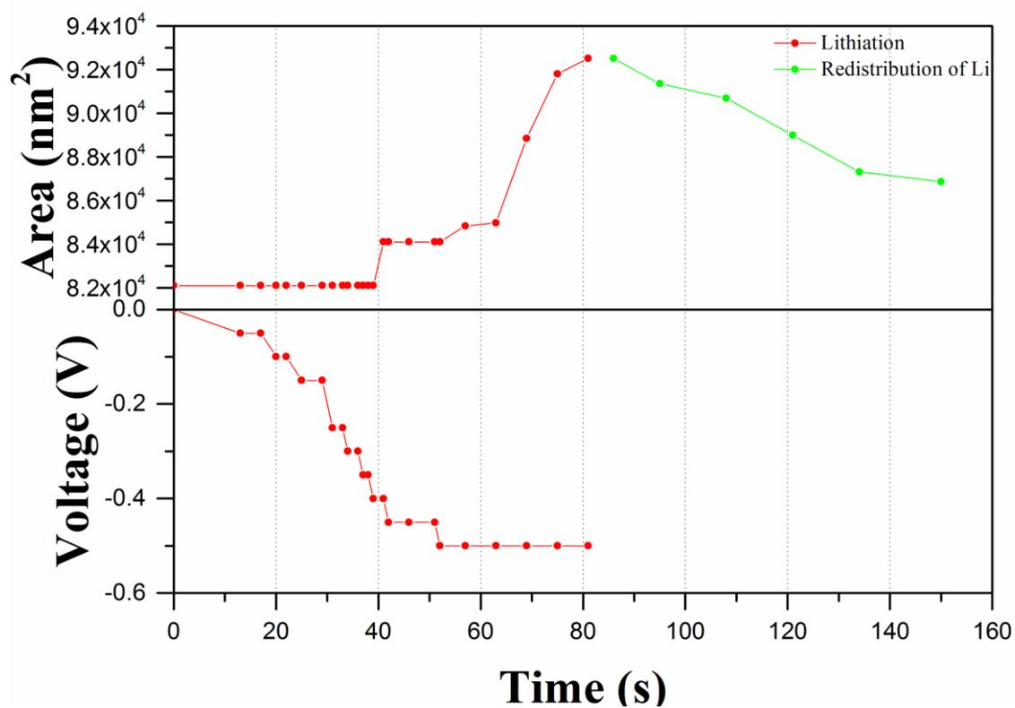
**Figure S5.** Expansion and contraction of a Si nanoparticle cluster during lithiation and subsequent redistribution of lithium. The plots show the area of the cluster measured from TEM micrographs and the corresponding applied bias voltage as a function of time.
