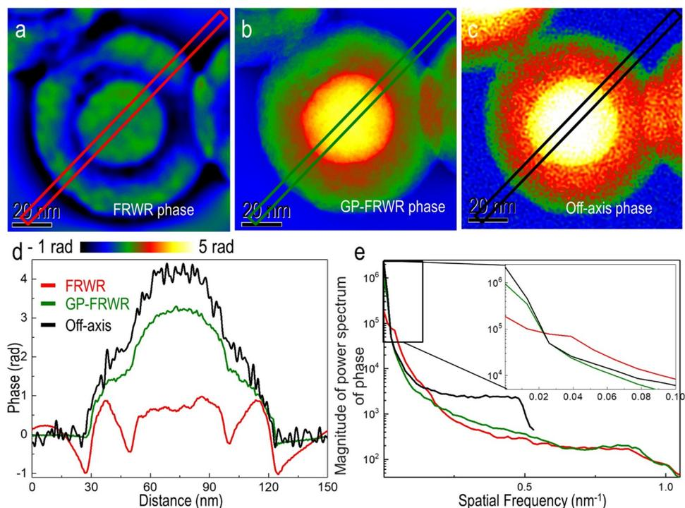
**Figure 1.** Phase images of Fe-filled C nanospheres were reconstructed using (a) FRWR, (b) GPFRWR, and (c) off-axis electron holography. (d) Line profiles extracted from the three phase reconstructions. (e) Radially-averaged power spectra of the three phase images.
