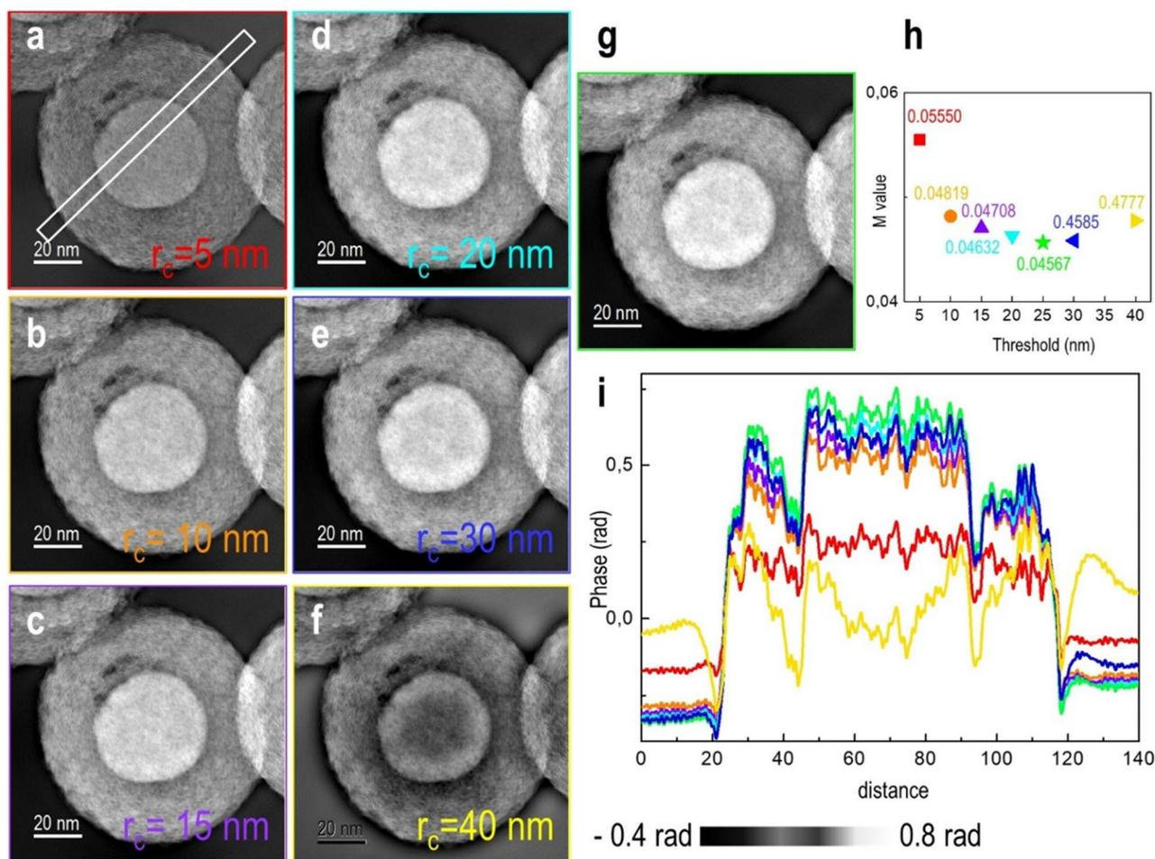
**Figure 2.** Phase images of Fe-filled C nanospheres reconstructed using (a) 5, (b) 10, (c) 15, (d) 20, (e) 30, (f) 40, and (g) 25 nm threshold values. (h) Threshold vs.  $M$  value (mismatch between simulated and experimental images). (i) Line profiles of (a)–(g) from the region marked in (a).
