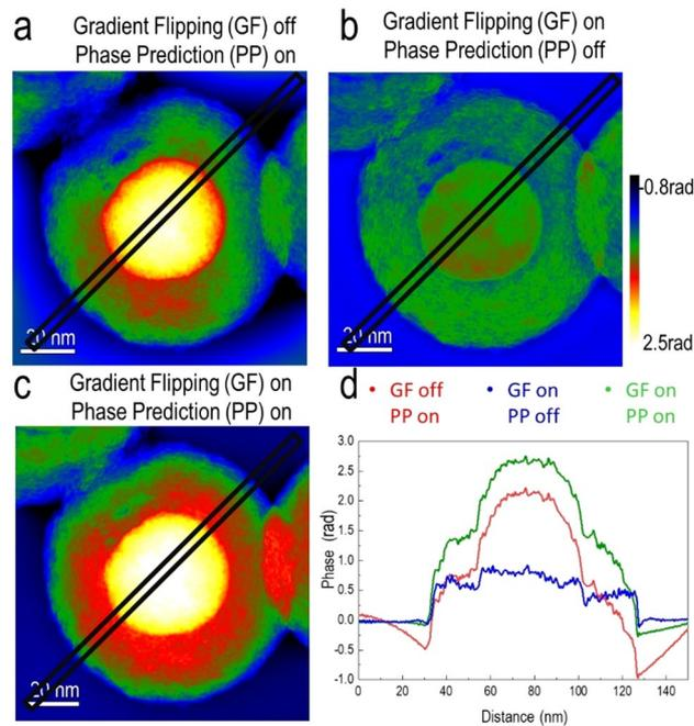
**Figure 4.** Comparison between individual and combined effects of gradient flipping and phase prediction. **(a)** Phase reconstruction with gradient flipping (GF) off and phase prediction (PP) on. **(b)** Phase reconstruction with GF on and PP off. **(c)** Phase reconstruction with GF on and PP on. **(d)** Line profiles extracted along the lines marked in the phase maps.
