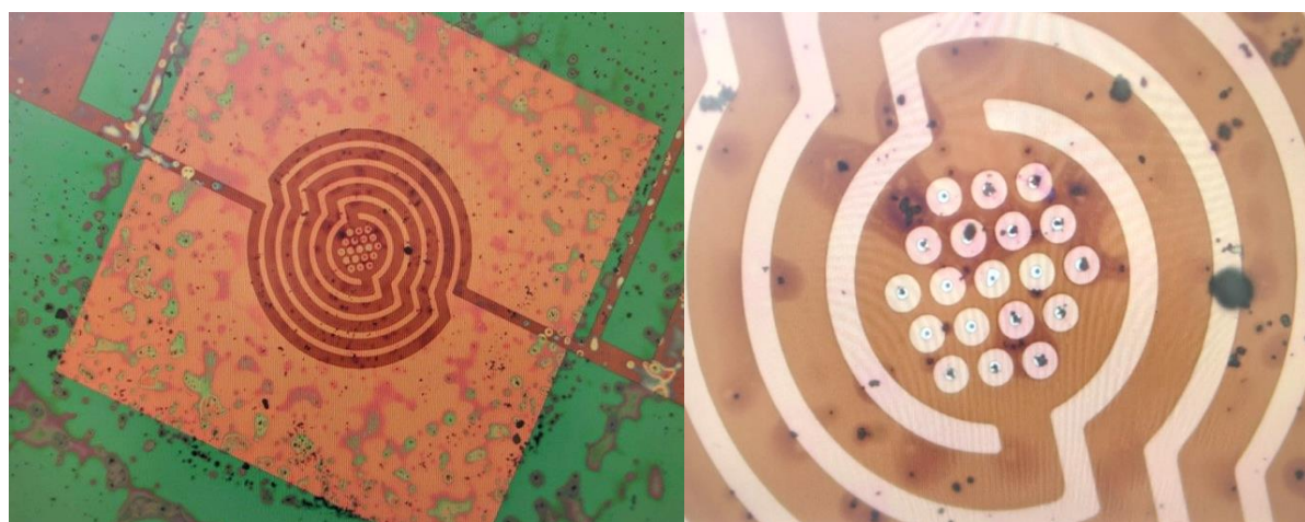
Figure S14: Optical microscopy image of a MEMS heating chip (Norcada Inc., Edmonton, Canada). Left: heating spiral with contacting, 5x magnification. Right: 50x magnification of SiN-windows in the centre of the heating spiral. The supported Pd(NO 3 ) 2 /ZnO specimen is visible as dark particles positioned on the windows.
